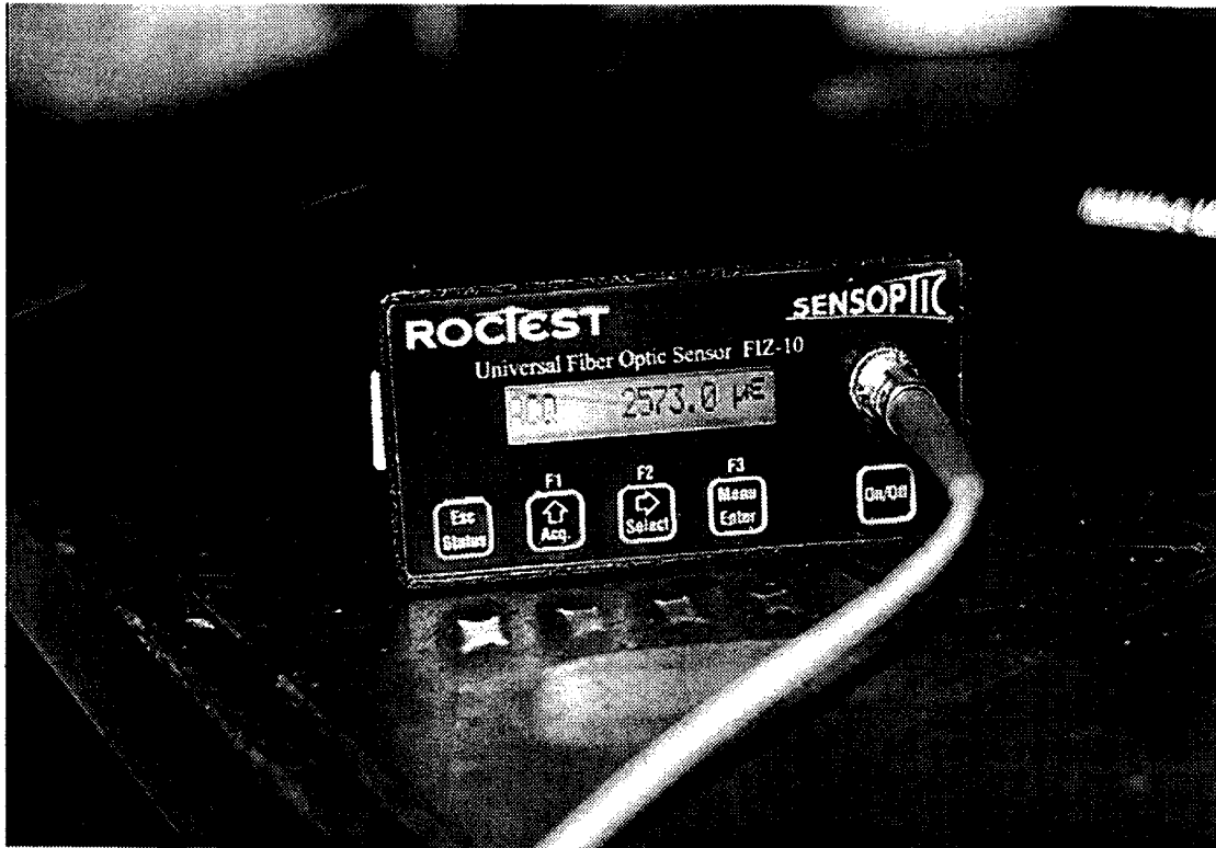
Figure 3-47: FIZ 10 demodulation unit for Fabry Perot sensors
