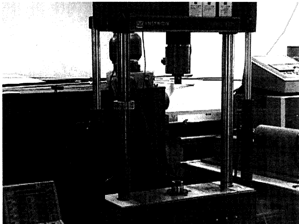
Figure 3-43: Instron machine used for tension loading of pultruded tendons
