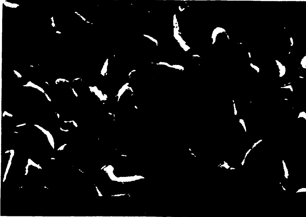
Figure 4-30. SEM micrograph of the same area as Figure 4-21 after the devitrification treatment.
