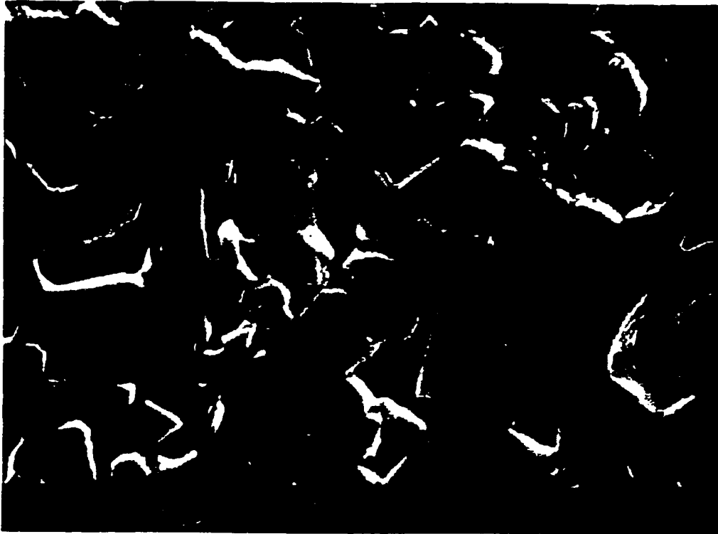
Figure 4-32. Micrograph of polished CAS surface after devitrification.
