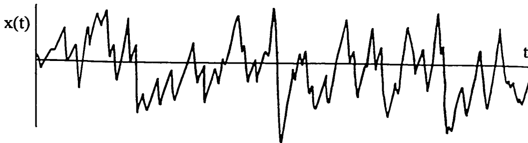
Figure A.2 Realization of a Random Process
