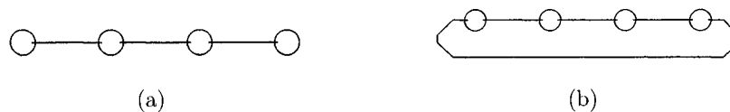
Figure A.6: (a) A simple array. (b) A ring formed by joining the first and last node of the array.
