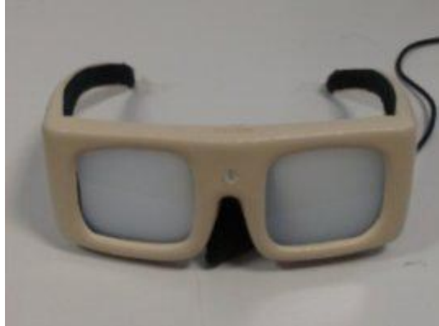
Figure 4. The PLATO translucent glasses fitted with a pair of LCD lenses that can be made opaque or transparent by the control of a switch.
