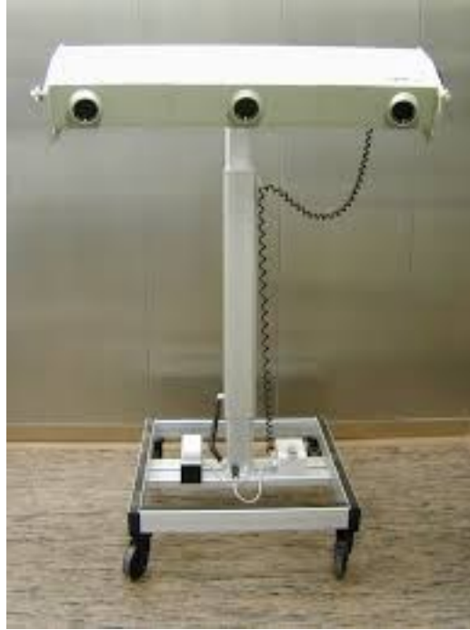
Figure 3. The three infrared detecting cameras of the Optotrak 3020 3D motion capture system.
