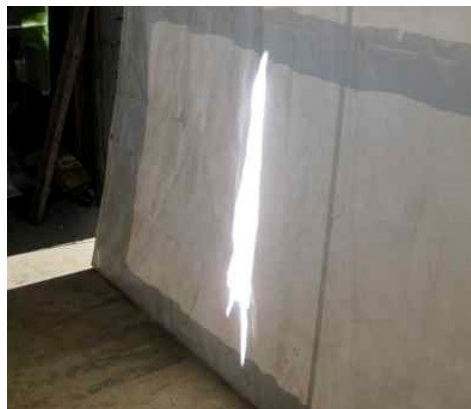
Figure 3-2. Focus image resulting from single 4'x8' reflector of 5' focal length constrained about its 8' edges with outermost 12.5% of reflector covered, showing much improved line focus.
