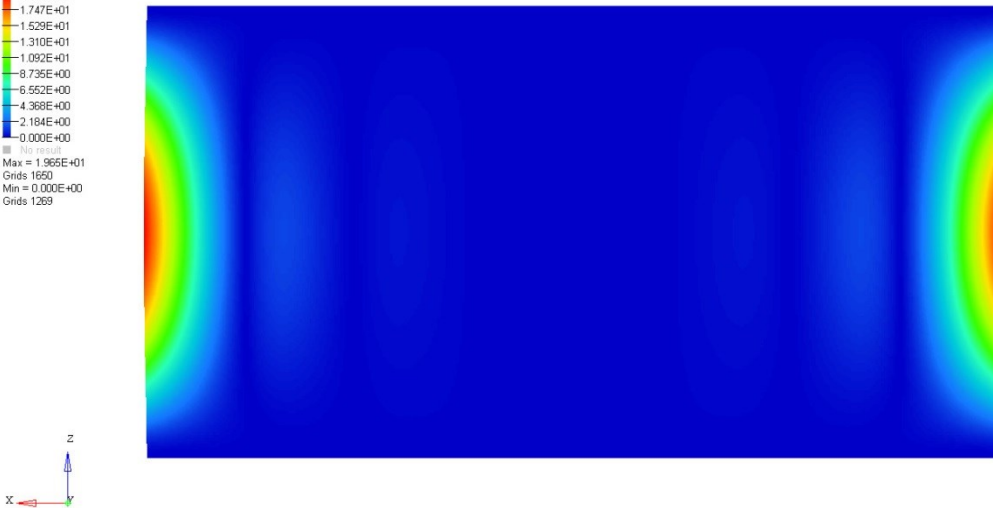
Figure A-14. Model 14: 0.29766 mm thick aluminum plate, fully constrained along two 8' lengths.
