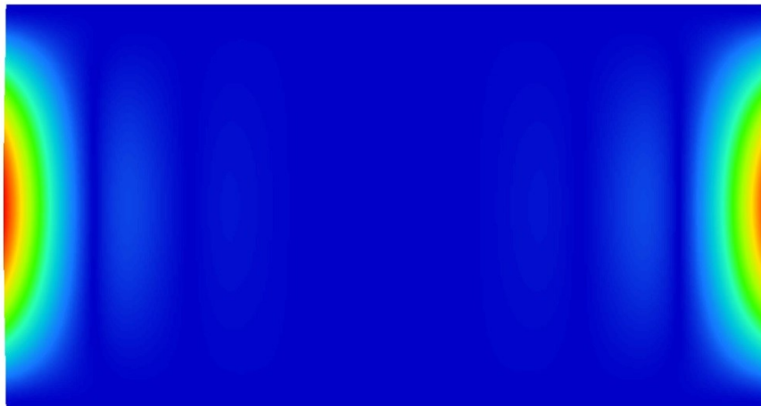
Figure A-4. Model 4: 0.29766 mm thick steel plate, fully constrained along two 8' lengths.
