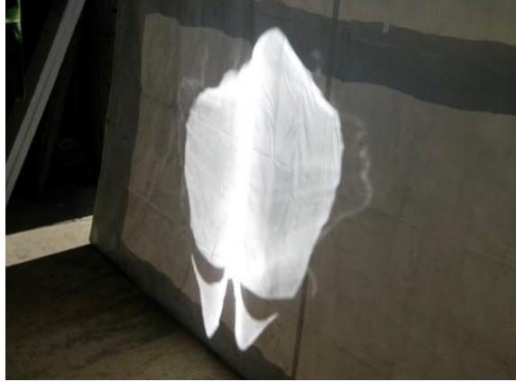
Figure 3-1. Focus image resulting from single 4'x8' reflector of 5' focal length constrained about its 8' edges, showing "hamburger buns" effect.
