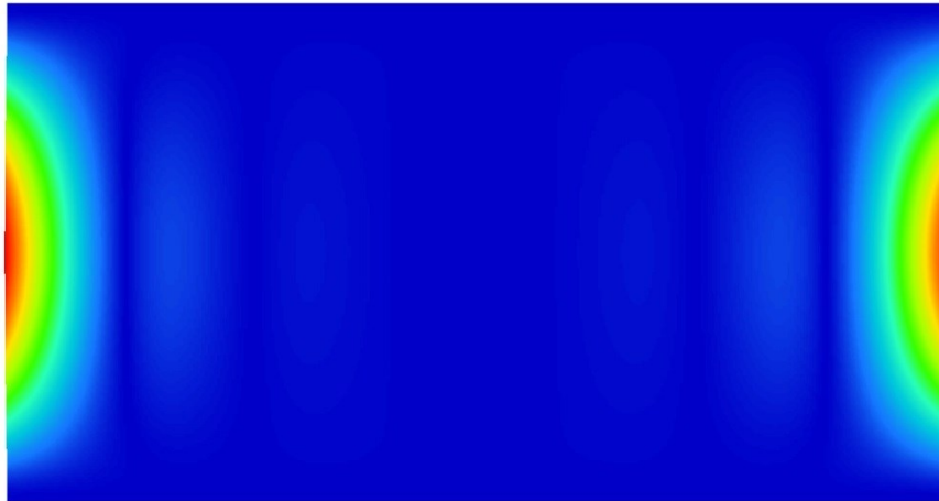
Figure A-3. Model 3: 0.39688 mm thick steel plate, fully constrained along two 8' lengths.
