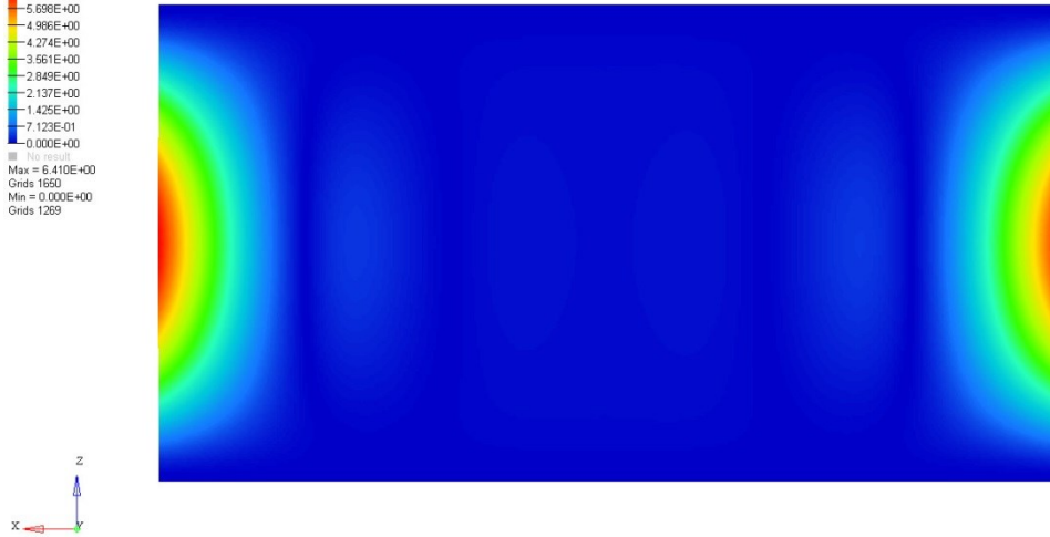
Figure A-10. Model 10: 0.79750 mm thick aluminum plate, fully constrained along two 8' lengths.
