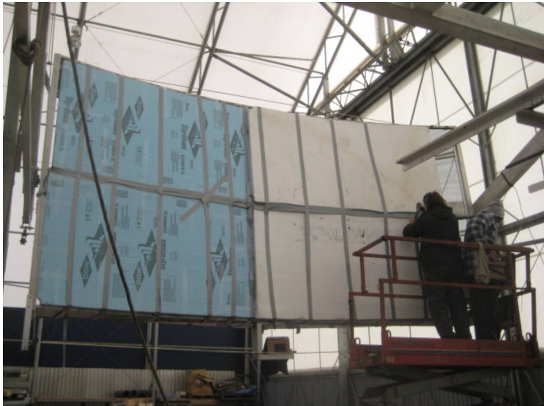
Figure 3-8. Gamma II prototype with all secondary reflectors covered in non-reflective Styrofoam except for final 1' of secondary reflectors #2, and #4 revealed, allowing for isolated observation and comparison of different stiffeners.
