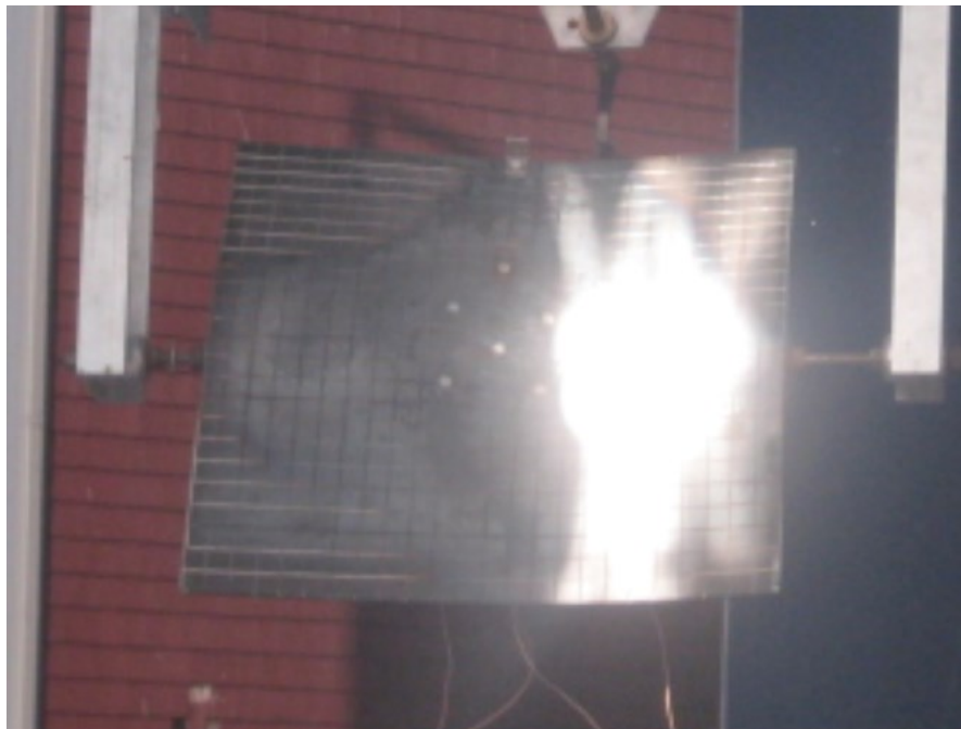
Figure 3-7. Gamma II focus image with all secondary reflector ends covered.
