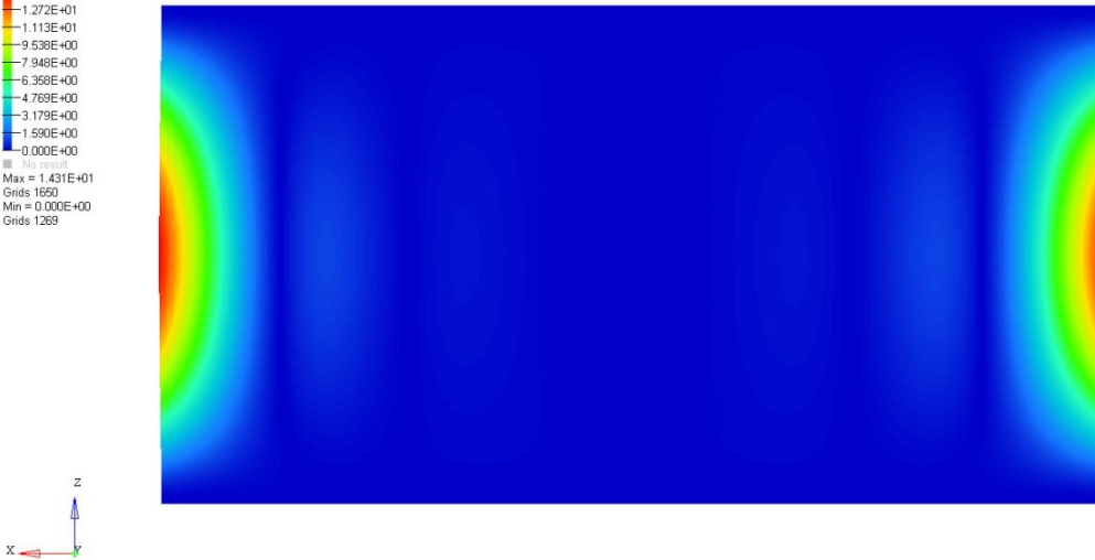
Figure A-13. Model 13: 0.39688 mm thick aluminum plate, fully constrained along two 8' lengths.
