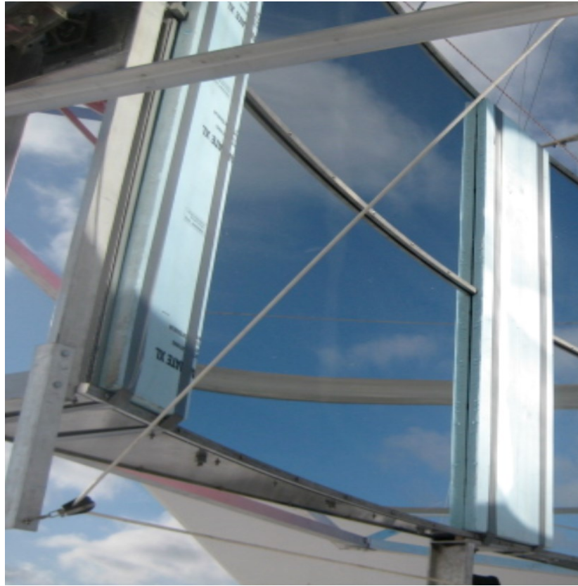
Figure 3-6. Gamma II prototype with final 1' of each secondary reflector covered in non-reflective Styrofoam.
