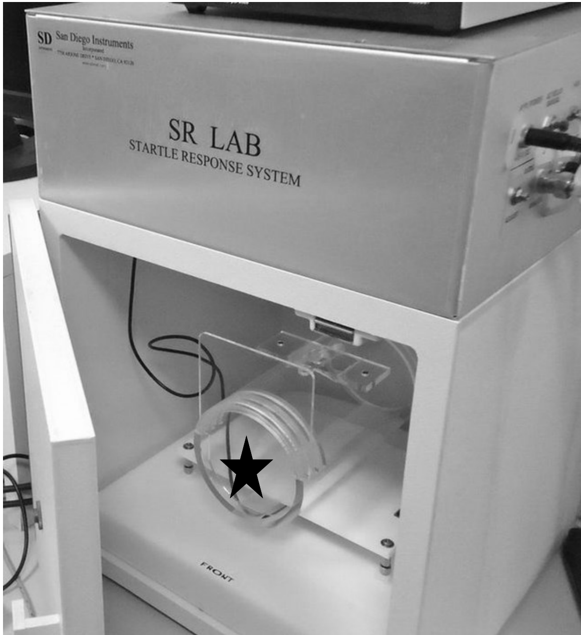
Figure 2.4. Photograph of the apparatus used for measuring sensorimotor gating (PPI) and startle-related variables.
