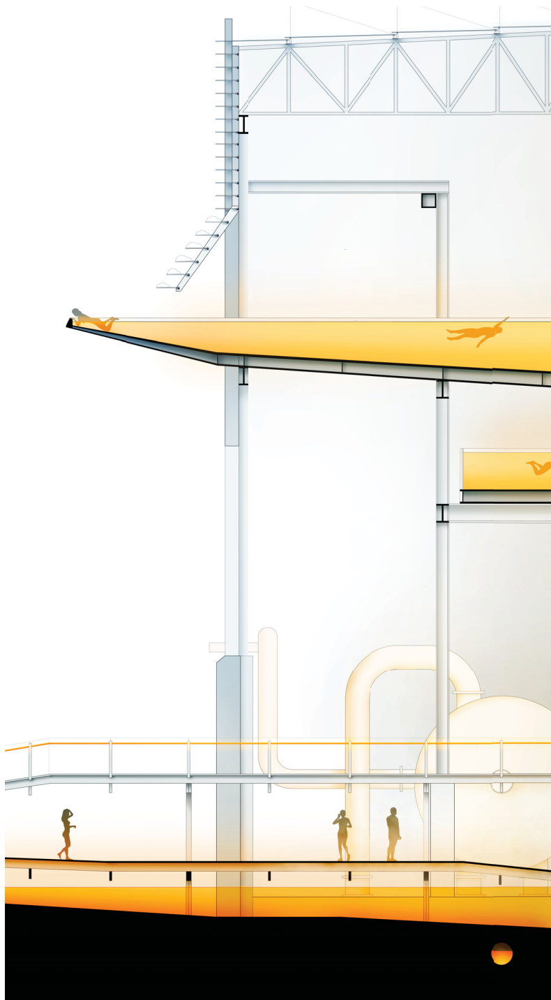
Section through the void in the boiler hall's facade and the suspended bath that emerges from within
