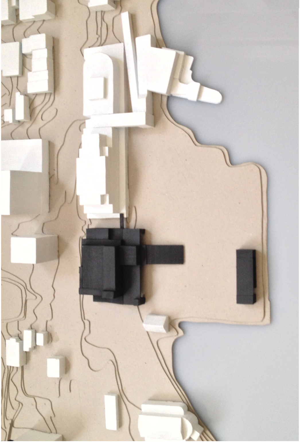
Site model showing the placement and massing of the building and outdoor stage on the site.
