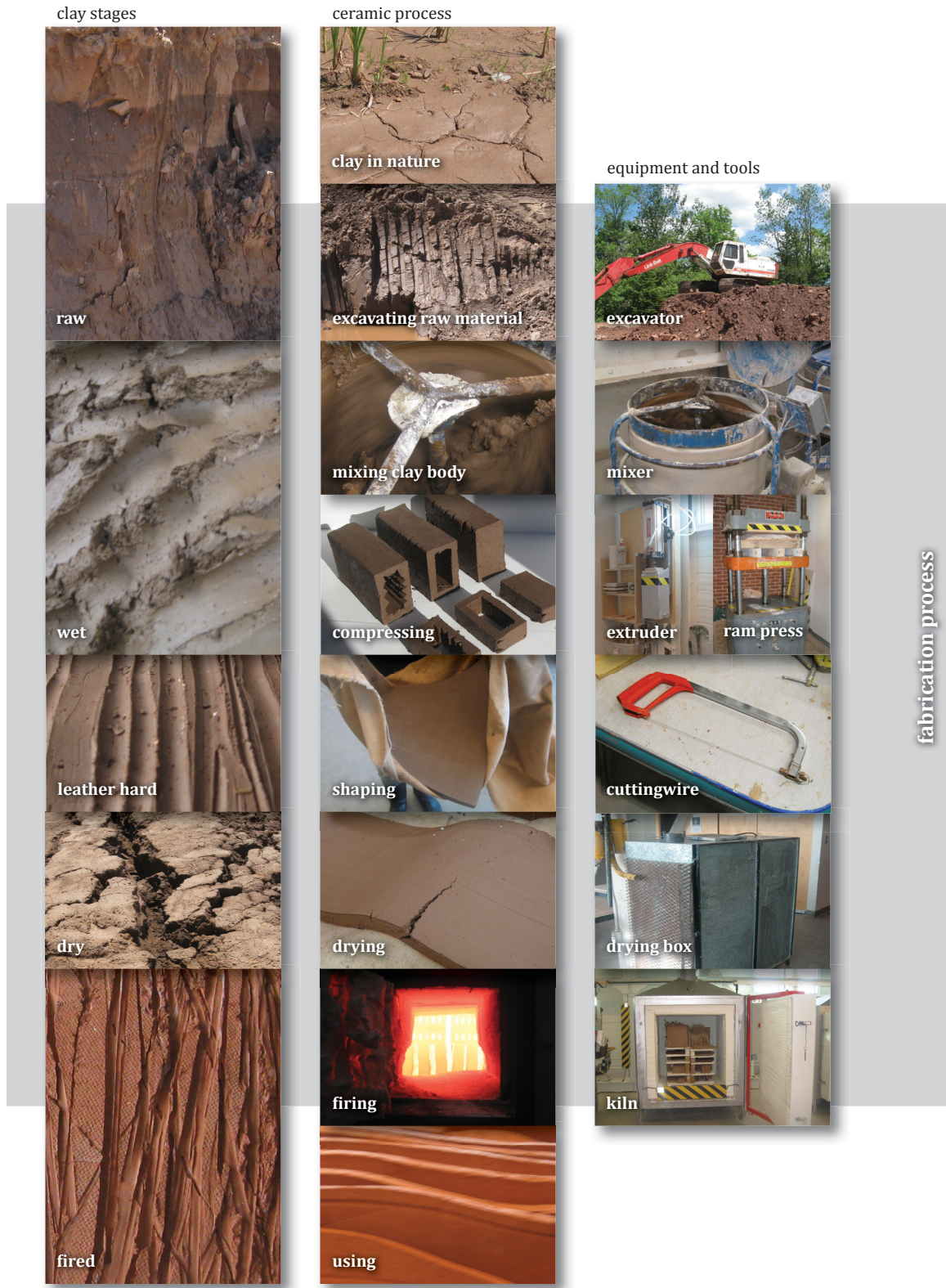
Photographs of ceramic process, illustrating the relationship between clay stages and the sequence of action and tools
