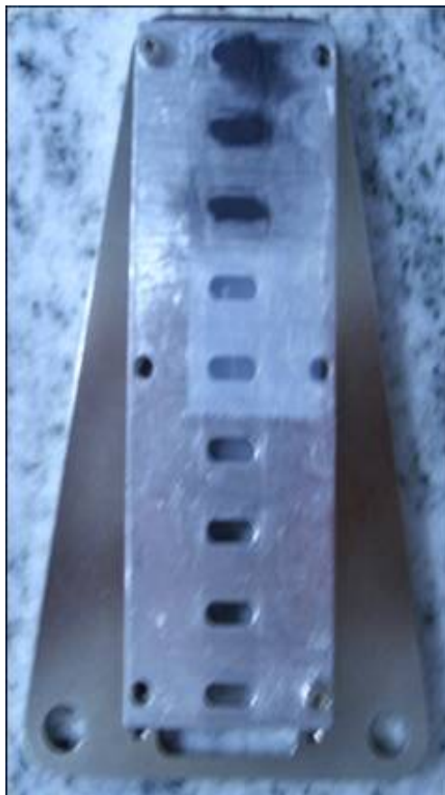
Figure 2.6 The carbon holder attachment with three samples loaded. Adhesive tape covers the front and back of the samples. The holder is screwed on to a triangular-shaped metal attachment that slots directly into the NanoSTAR sample stage.
