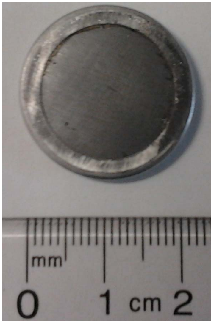
Figure 2.4 The transmission-mode in-situ coin cell viewed from the can, with scale.
