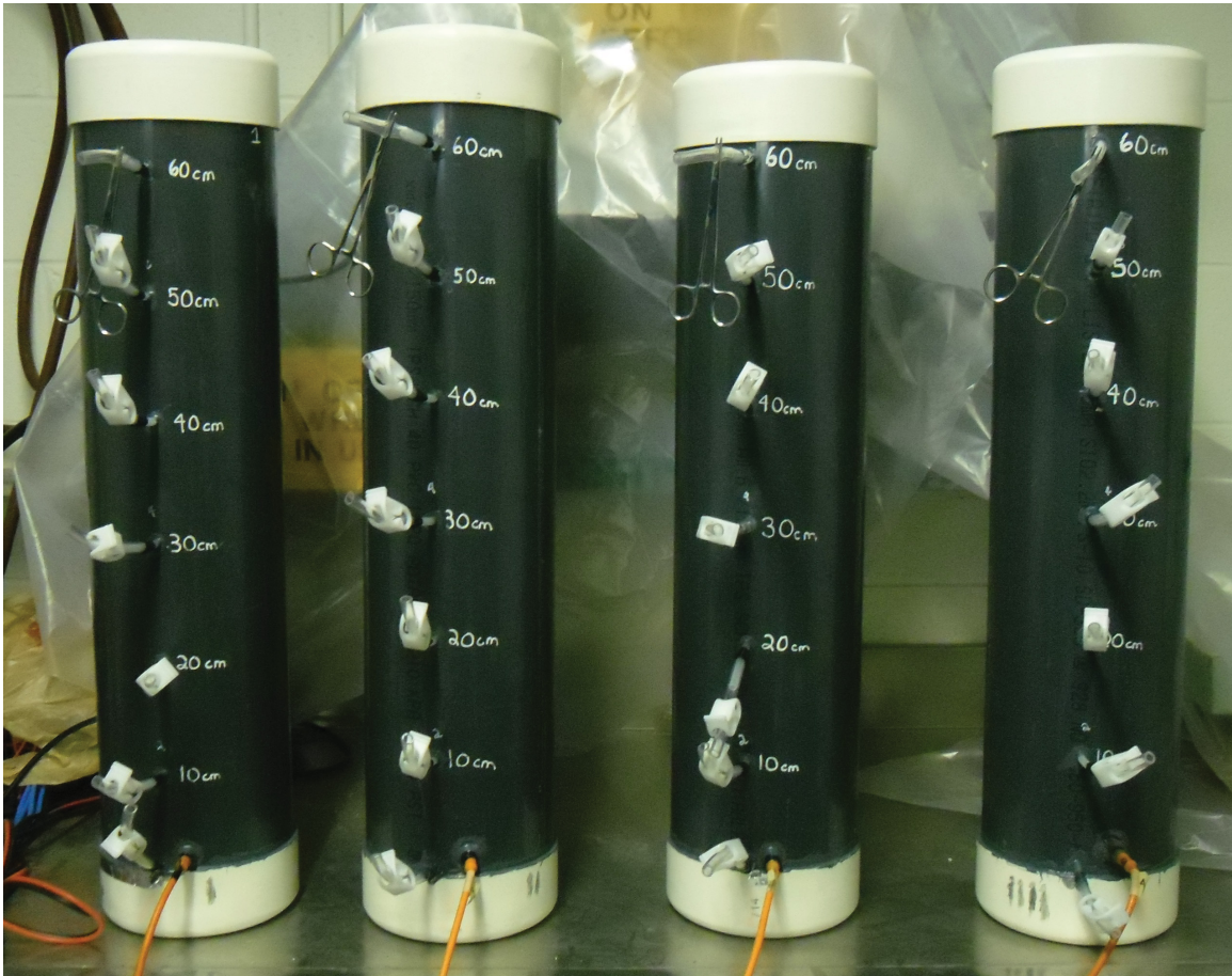
Figure 3.6: Columns 1 through 4 (left to right) filled with local tills and bedrock cores. Note the tubing extruding every 10 cm up the sealed columns. The cracks around the tubing holes were filled with Cole Parmer Very High-Peel Strength Epoxy. The height differences between the columns are a result of the thickness of the respective bedrock cores.
