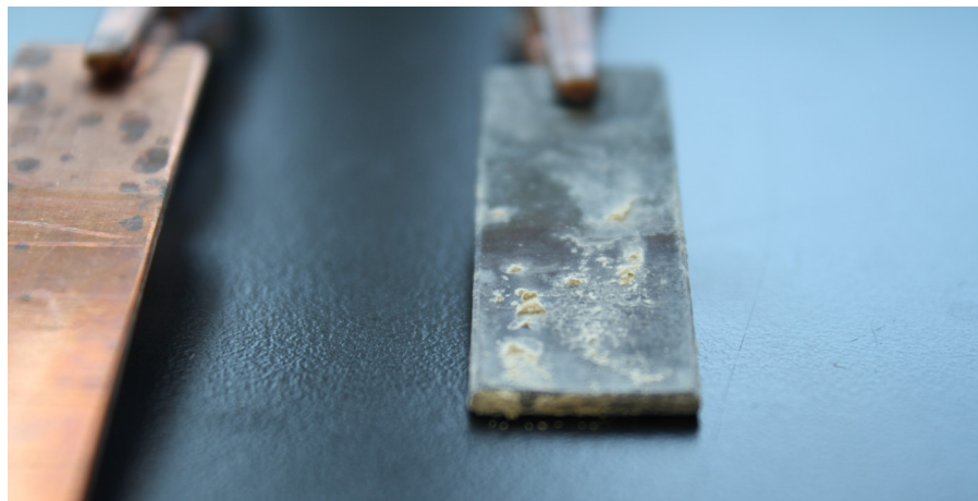
Figure 4.26 – Post-experiment copper and lead coupons from water condition OP(20)/pH7.3/DIC(7). White corrosion tubercles are extending from the lead surface.
