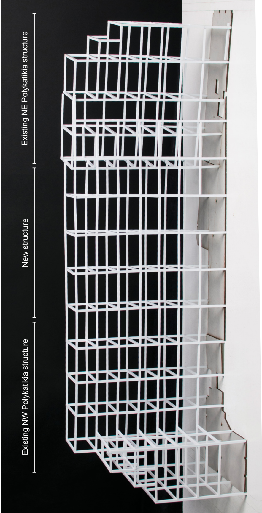
Figure 45: Structural study of creating a new architecture based on the familiar post and beam technology. Modelled at 1:100
