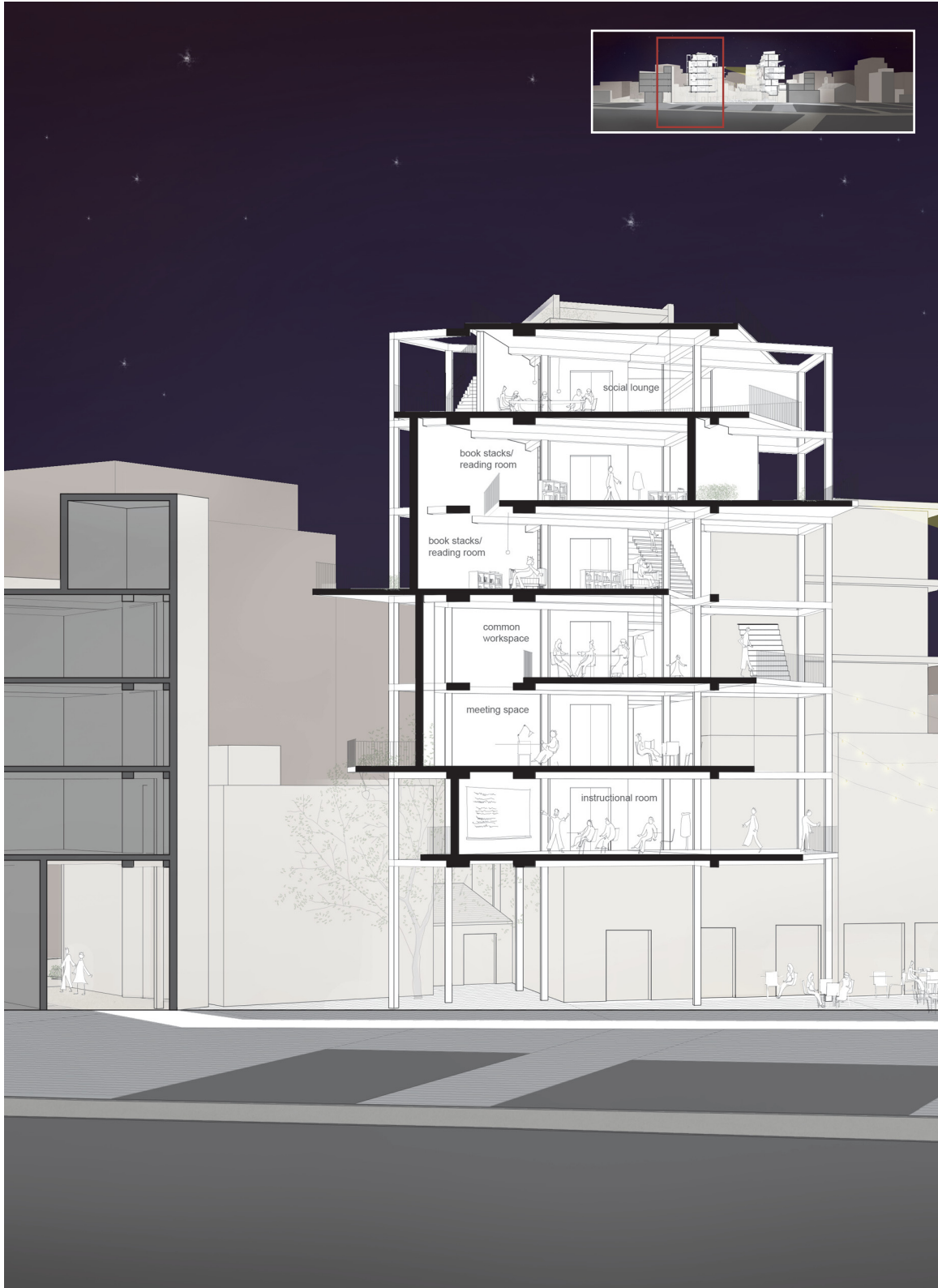
Figure 107: Transverse section of tower complex. To the left is a stoa providing connection to platea Iron.
