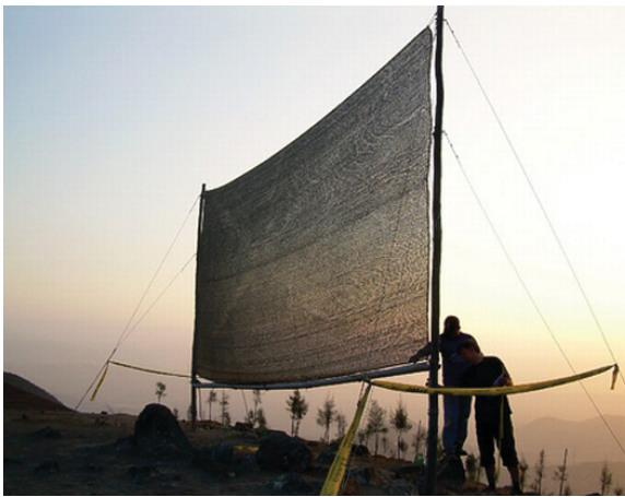
Passive fog collector (Lummerich 2010)
