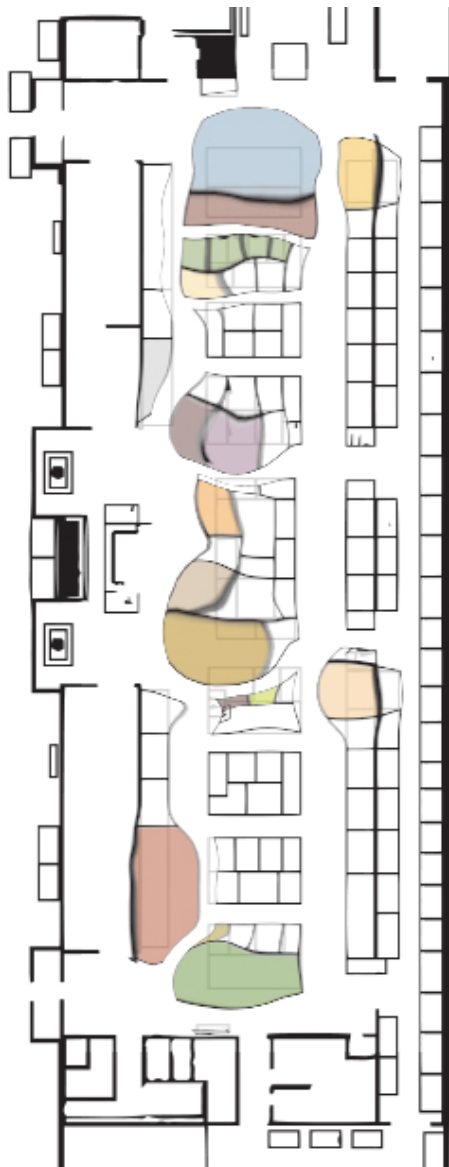
Stall influence diagram showing where people tend to gather and how it affects flow.
