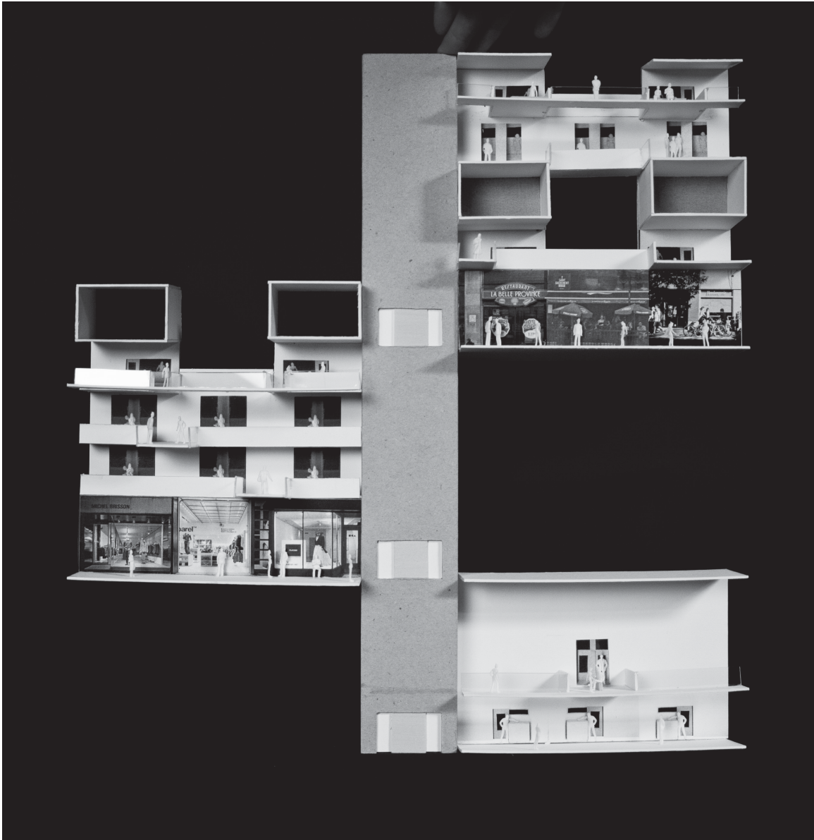
Fig. 40 1:100 Sectional model used to study the interior form of different “streets”, This conceptual model shows a gradient of activity from the quietest street at the bottom right to the busiest street at the top right.
