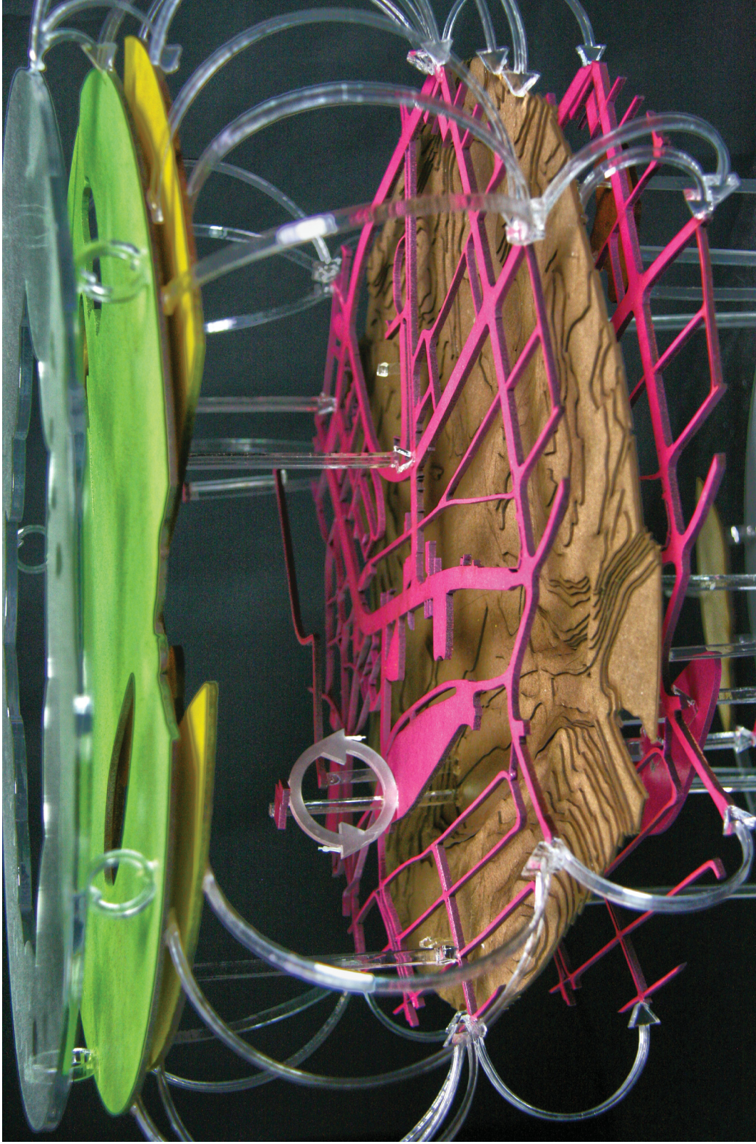
Detail photograph of systems model showing location of RCOC and dry pond parking lot and system layers from top to bottom - atmospheric reservoir, vegetation, roofs, RCOC, green swale, roadways, topography, wetlands, Ominik Marsh, Clear Lake and the aquifer
