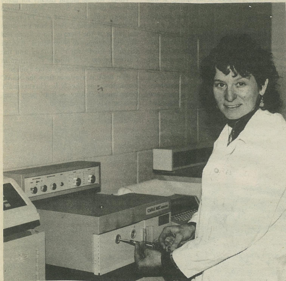
Karen Stratton ('75) is shown working with a Carle gas chromatograph with flame ionization detector.
