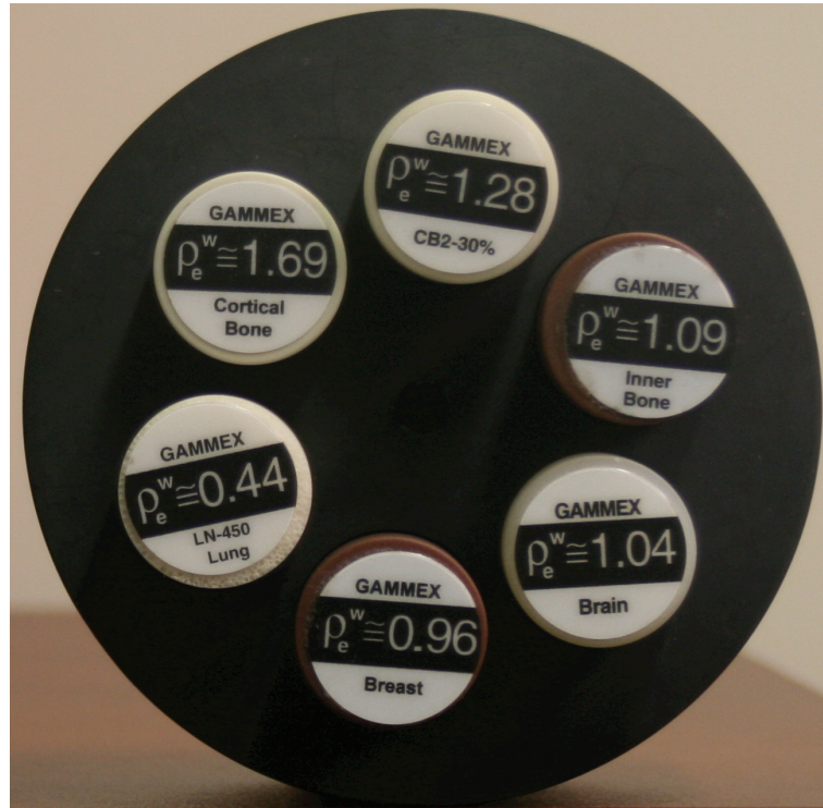
Figure 7.10 The CNR phantom used for CBCT with the tissue substitute materials.
