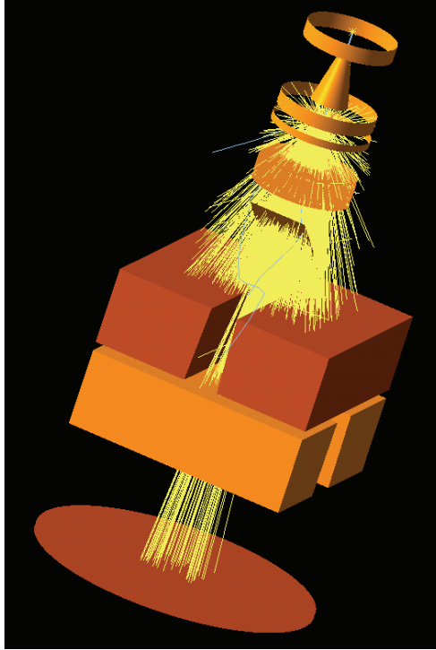
Figure 7.4 Monte Carlo simulation of the Varian 2100EX linac with the therapeutic target and flattening filter removed and a carbon target placed at the level of the flattening filter
