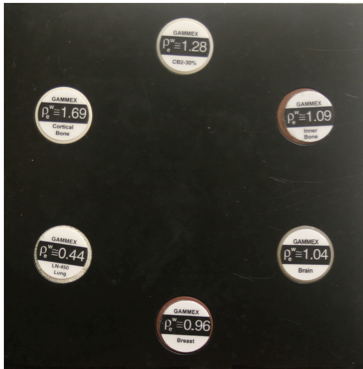
Figure 7.5 The CNR phantom with tissue equivalent inserts.
