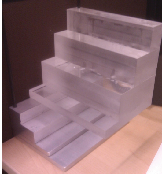
Figure 4.1: Cross-wedge phantom for calibrating empirical DXA equations. Aluminum simulates bone under x-ray, acrylic for soft tissue.
