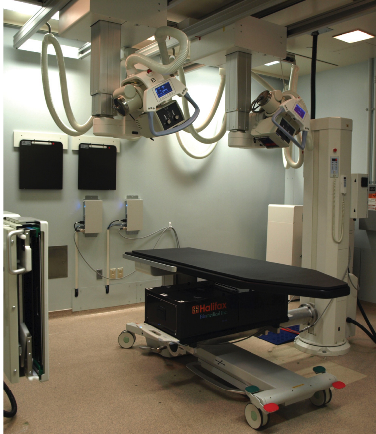
Figure 2.1: SR Suite at the Halifax Infirmary. Dual x-ray heads at a 30^\circ angle to vertical and a calibration box (HalifaxBox007, Halifax Biomedical Inc., Mabou, NS, Canada) under the table which houses the RSA spatial reference beads and the digital detector plates.
