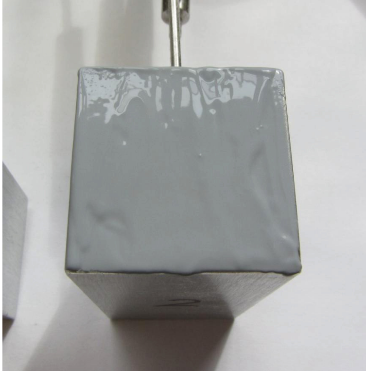
Figure 4.2 Photograph of a Tgrease 880 sample after being initially applied to the meter bar.
