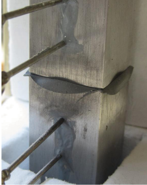
Figure 4.5 Photograph of a Tflex 720 sample after testing while still in the interface
