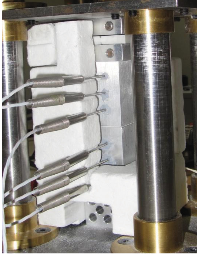
Figure 2.6 Photograph of partially assembled insulation blocks
