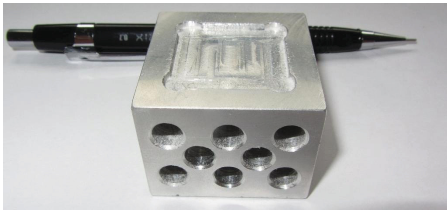
Figure 2.4 Photograph of the heater block and guard heater
