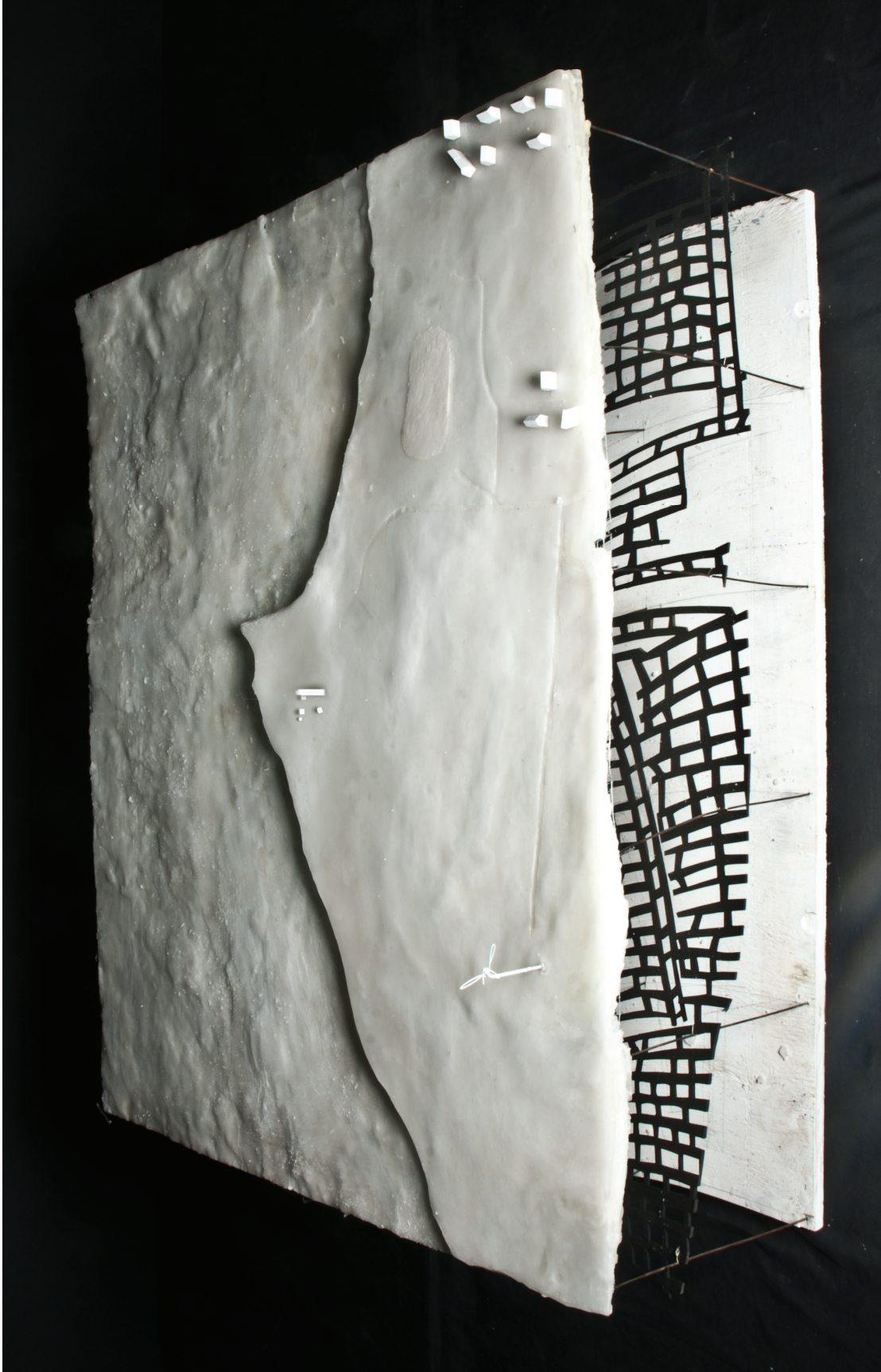
Concept Site Model. Wax + wire topography supported by metal struts on wood base. Mines in black card suspended. Scale 1:1000.
