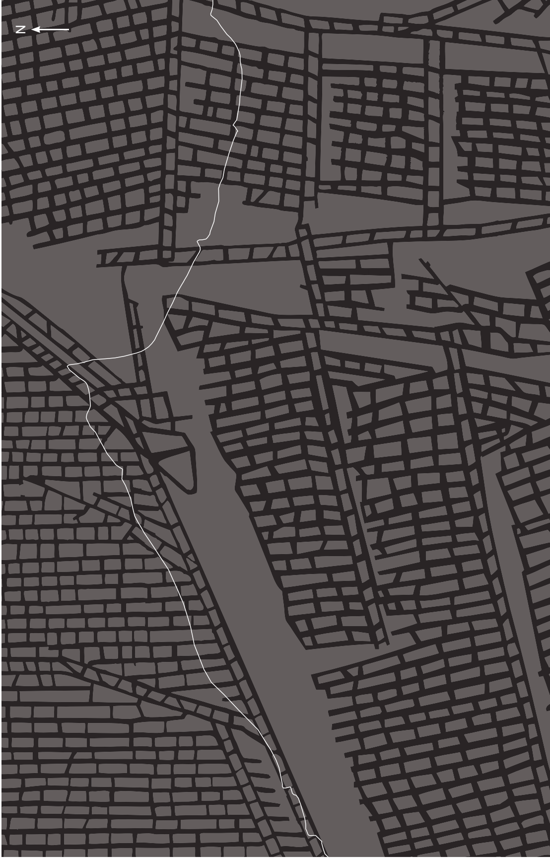
Plan of the Phalen Seam, 201 meters below Colliery 1B+26. The mine extended north over 5.6 kilometers under the ocean. Scale 1:5000.
