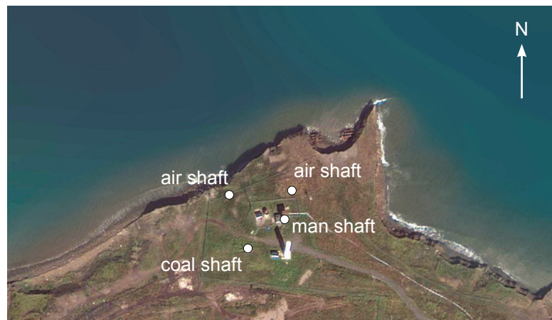
Former site Colliery 1B+26. Scale: 1:5000.
