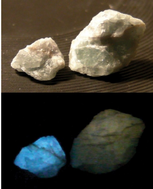
Figure 2-37: Thermoluminescence of a fluorite (chlorophane) that emits light when heated. Image extracted from (Encyclopædia Britannica Inc., 2012)
