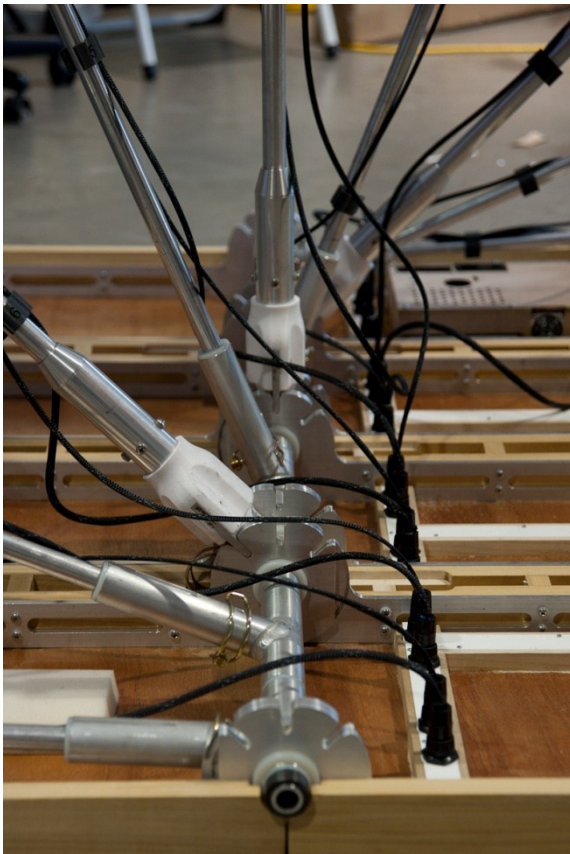
Figure 3-19: A close up of the central axis with assembled poles. The central axis lies in the wooden platform and the backdrops structure can be disassembled to fit inside the platform for transport
