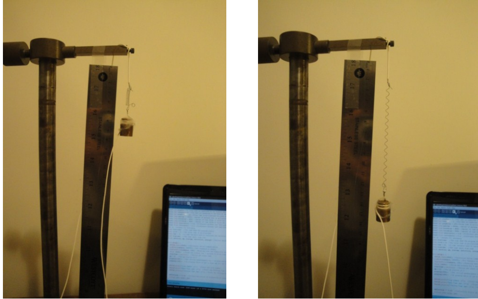
Figure 6-26: Each time the wire was in its austenite phase (Left) and martensite phase (Right), the bias mass's position on the ruler was recorded.
