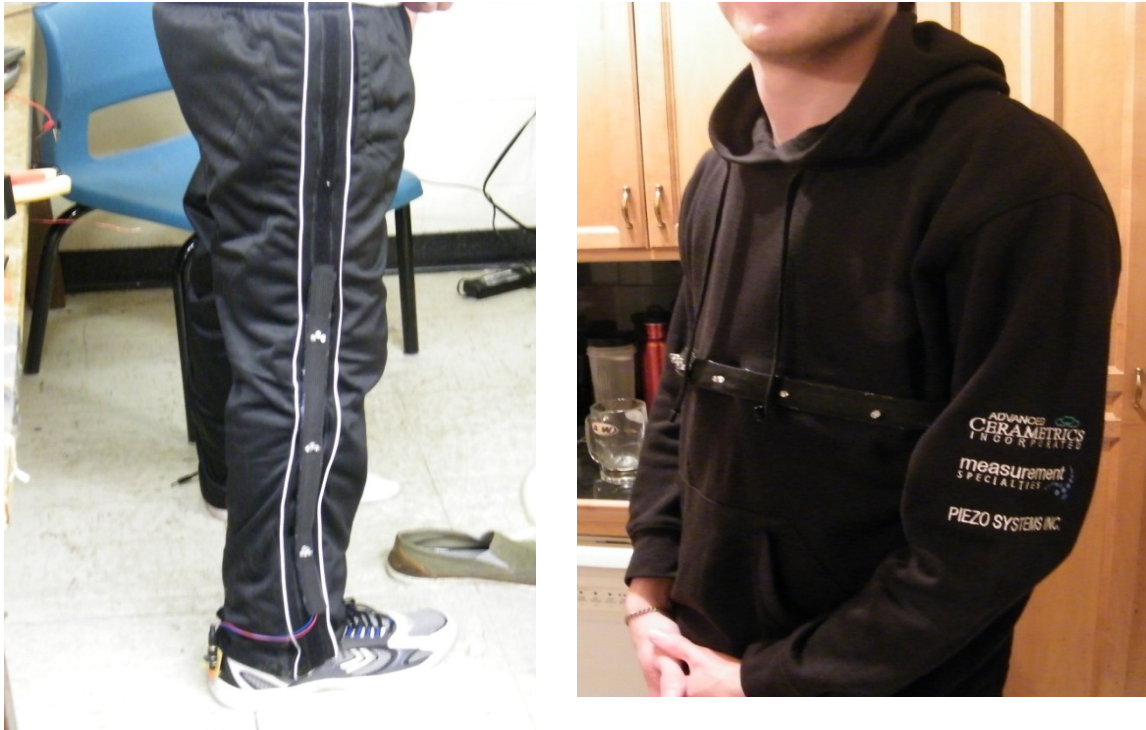
Figure 3-27: The Human Powered LED Jogging Suit. (Left) The pants have LEDs powered by piezoelectric inserts in the shoes and are sewn into the pants using conductive thread. (Right) the sweater has LEDs powered by electromagnetic inductive shakers located on the waist.
