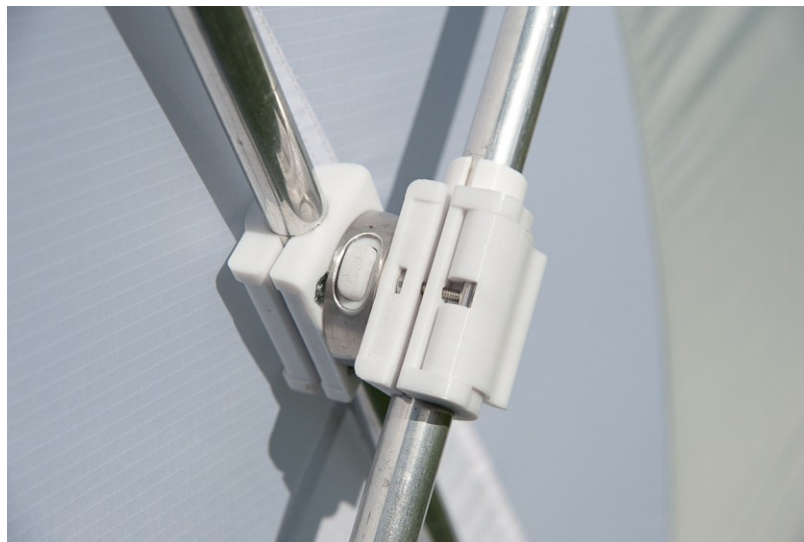
Figure 4-5: An aluminum ring was added to encase the mid section of the universal sliding joint and improve its structural integrity
