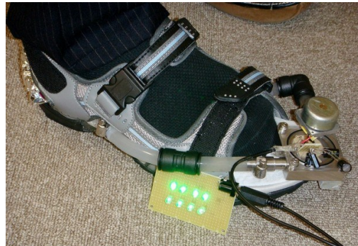
Figure 5-31: NTT Corp. developed shoes that uses water turbines to produce power. Image extracted from (Japan Probe, 2008)
