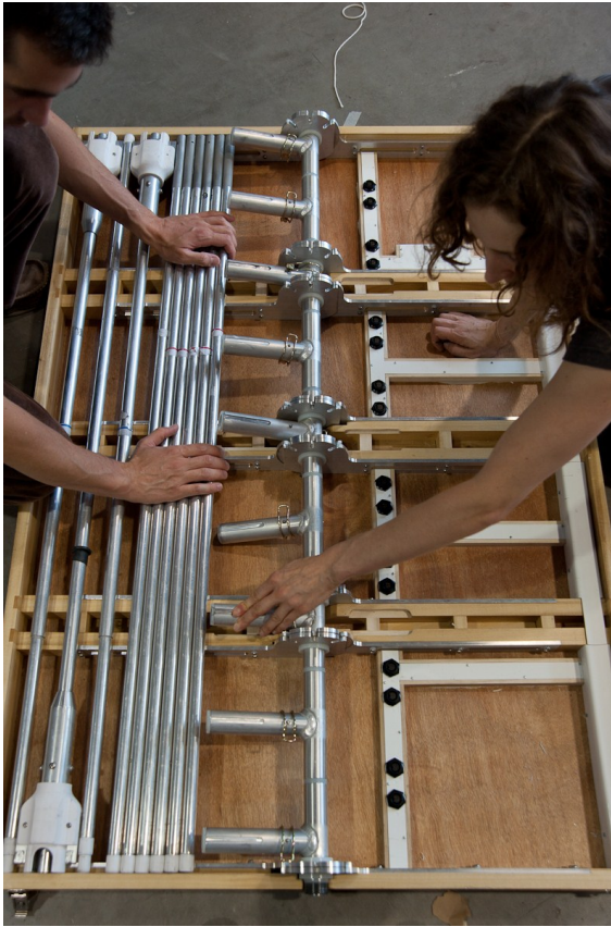
Figure 4-6: The Flamenco Backdrop has poles that collapse telescopically so that they can fit inside the Backdrop's platform/carrying case
