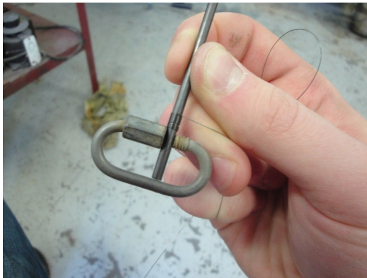
Figure 6-20: To constrain the Flexinol ® wire to a helical spring, one end of the wire was clamped to a rod, followed by tightly wrapping the wire around the rod, and constraining the other end with an additional C-clamp
