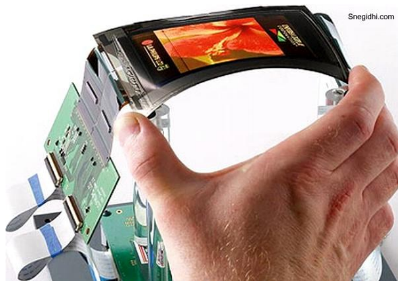
Figure 2-40: At the 2009 Society for Information Display in San Antonio, Samsung showcased their prototype Active Matrix OLED (AMOLED) screen. The new screen is much more flexible than its predecessors and has a response time that is 1000 times faster than a standard LCD. Since then, this technology has been used in more than 50 cell phone, music player, and game console models (Snegidhi.com, 2009)
