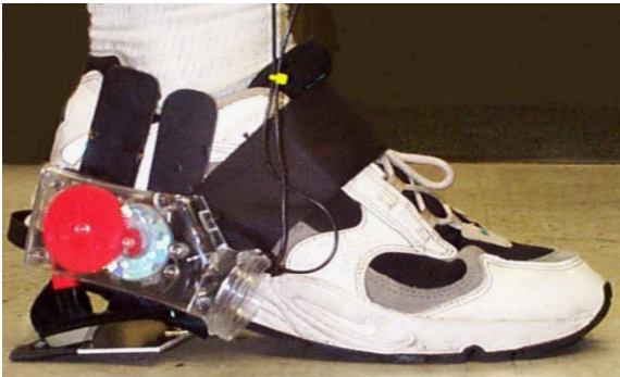
Figure 5-30: A Rotary Magnetic Generator completely embedded into the sneaker's sole (1999). Image extracted from (Responsive Environments Group-MIT, 2006)
