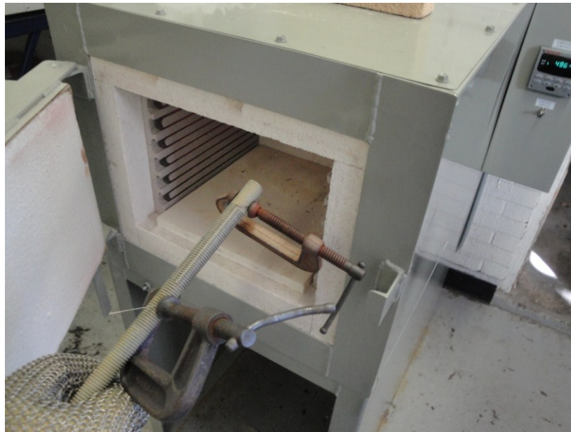
Figure 7-14: The Power Screw/Superelastic Spring Assembly was put in an Inferno™ oven for 25 minutes at a temperature of 500°C followed by a water quench
