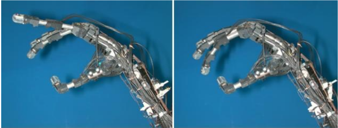
Figure 2-57: Due to their ability to directly respond to an electric field and their large deformation, researchers are looking into EAPs for artificial muscles. Image extracted from (Bar-Cohen, Artificial Muscles , 2011)
