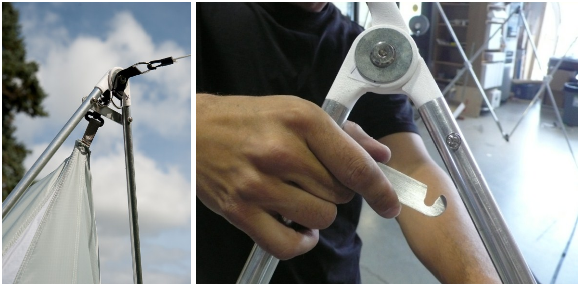
Figure 4-3: Adding hinged latches to the pivot joints not only locked them into place, but helped to suppress vibration and prevent twisting between adjacent links.
