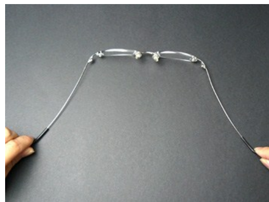
Figure 2-33: Superelastic NiTiNOL is used on eyeglass frames, enabling them to bend without permanent plastic deformation. Photo from (Rakuten Global Market, 2012)
