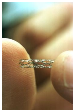
Figure 2-32: SMA's are used to make medical stents that expand when inside the human body. Photo from (Nixon, 2008)
