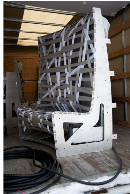
Figure 4-20: Additional material was added to the seat where it connects to the structural frame
