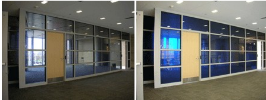
Figure 2-20: SPD Smartglass has the ability to instantly darken from 50% down to 1% light transmission for video conferences and presentations and can also regulate the amount of heat coming into the building while blocking 99% of harmful UV rays as well. Photo extracted from (Innovative Glass Corporation, 2006)
