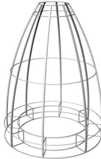
Figure 4-15: The Original Warming Hut's Design. Structure and fabric (left) and structure only (right). The structure is composed of 8 vertical members, 5 horizontal rings, and seats all made from aluminum bar.
