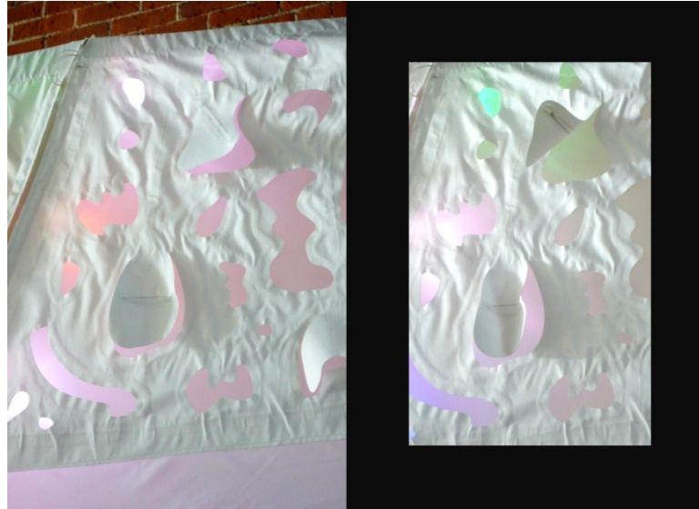
Figure 3-21: Fabric Flaps are actuated by SMA Springs and bias forced using Superelastic Nitinol. The left image shows two flaps in their resting state while the right image shows the flaps in their reactive state
