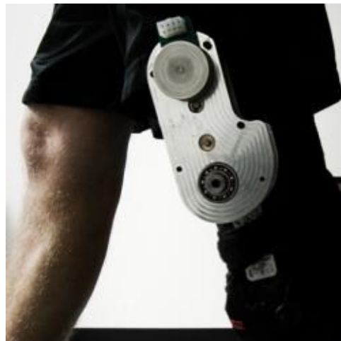
Figure 5-23: The Knee-Mounted Generator by researchers at Simon Fraser University. Photo extracted from (Inman M., 2008)
