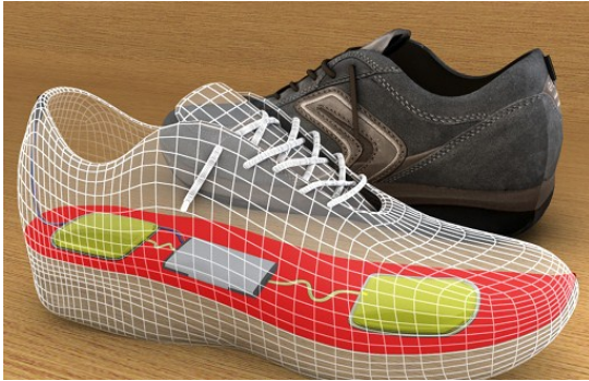
Figure 5-28: The energy harvesting shoe concept developed by InStep Nanopower using reverse electrowetting to generate electricity from human footfalls. Image extracted from (InStep NanoPower, LLC, 2010)
