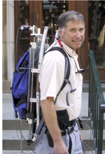
Figure 5-26: The Power-Generating Backpack attached to its inventor, Larry Rome. Image Etracted from (Lester, 2005)
