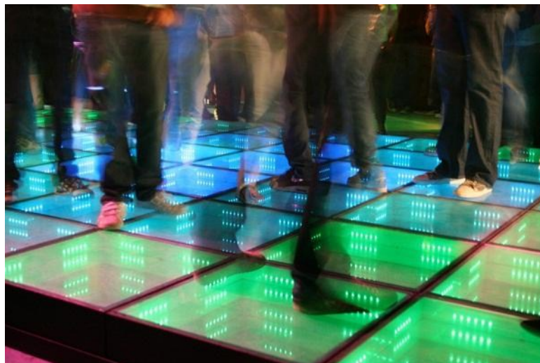
Figure 3-1: The Power Generating Dance Floor created by Enviu and Dutch architectural firm Döll. Image Extracted from (Zucker, 2011)
