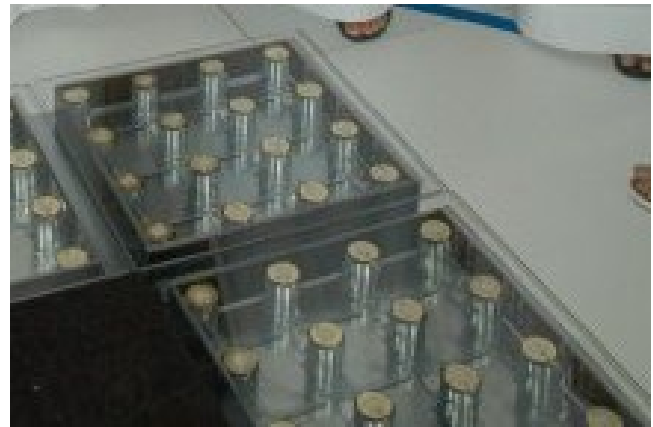
Figure B-4: (Left) Elizabeth Redmond presenting the 3 rd Generation POWERleap Prototype at the World Energy Summit in Abu Dhabi, UAE that took place between January 18-21, 2010. (Right) A closeup of the prototype shows that the third generation consists of 16 columns with piezoceramic discs. Image Extracted from (Gil, 2010)
