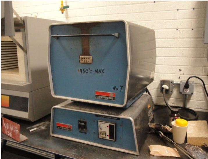
Figure 6-21: The wrapped wires were baked in a Lindberg™ oven (pictured left) at 500 °C for 10 minutes
