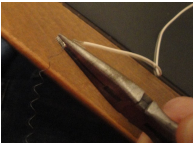
Figure 6-23: After going through the heat treatment, the springs were cut to their designated length and each end was crimped to an insulated electrical wire.
