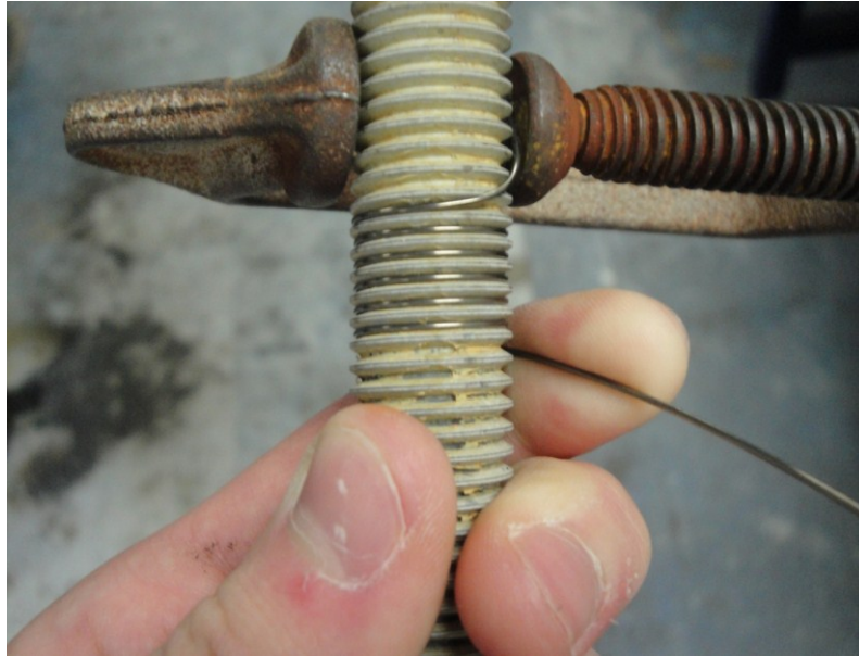
Figure 7-13: A C-clamp was used to constrain one end of the superelastic wire to the power screw. The wire was then wrapped around the power screw within the grooves before constraining the other end of the wire to the power screw.
