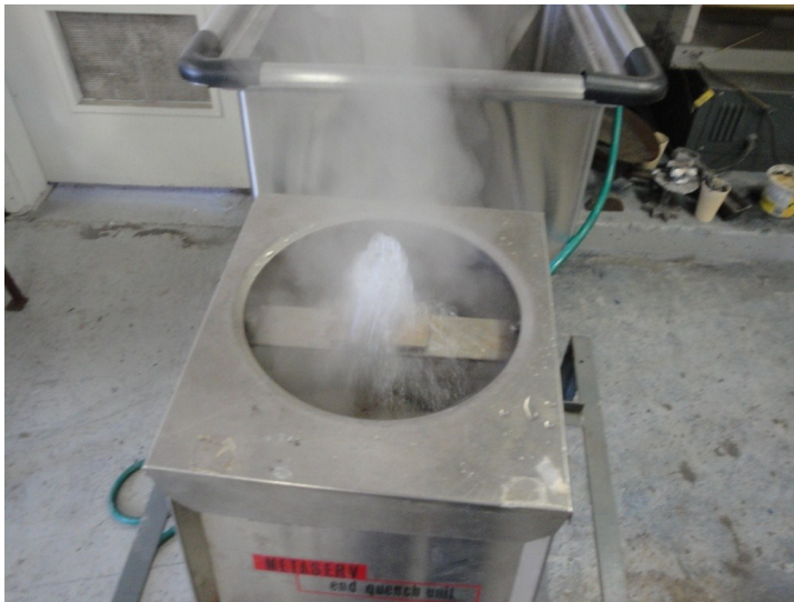
Figure 6-22: After heat treating, the wires were water quenched
