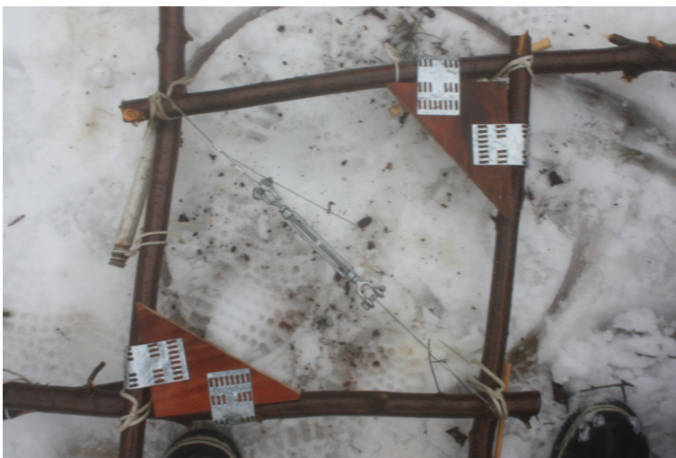
First iteration of the compression plates: Proved to be too small
