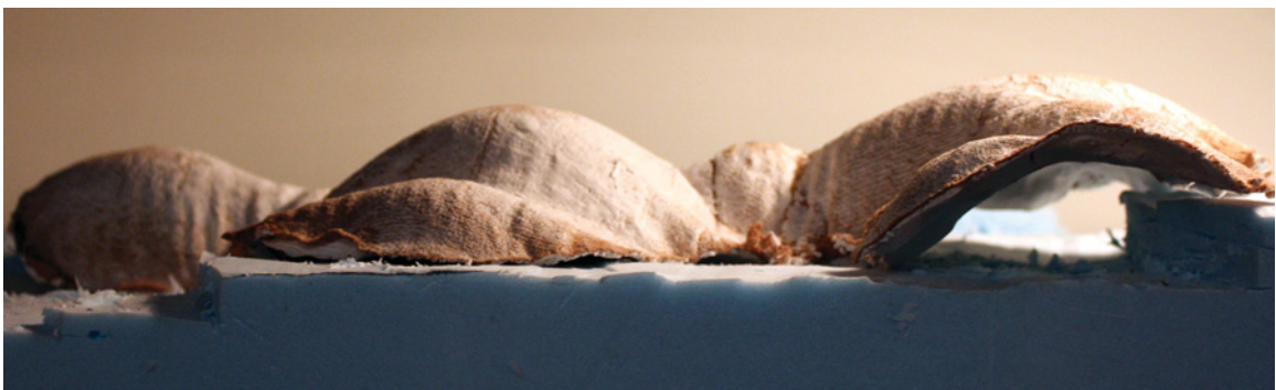
Design model - fabric and plaster. This model explores how the shell can negotiate the changing landscape by changing the support conditions of the suspended model.
