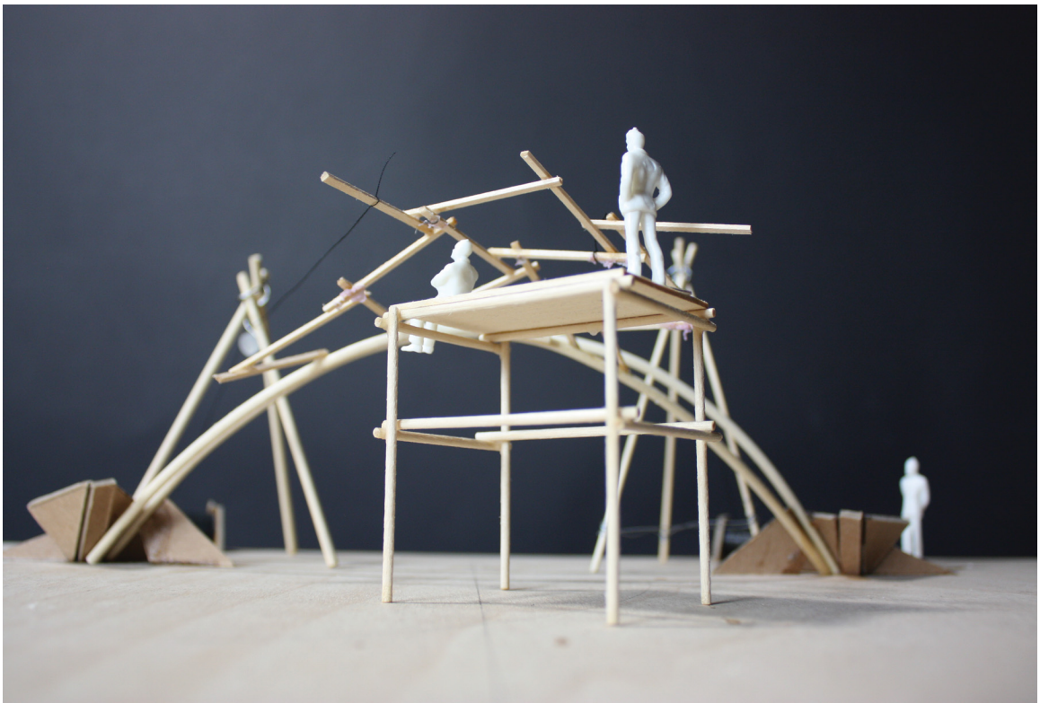
Photos of a model showing how the gridshell system will spring from the primary structure. Tension connections inspired by the tension connections in the network are used to hold up the system during construction, rather than letting it rest on scaffolding.
