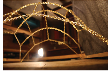
Hanging chain model that shows the ideal form of the shell
