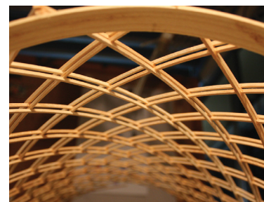
Gridshell structure study models.
