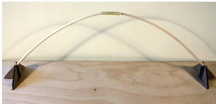
Bent wood three hinged arch
