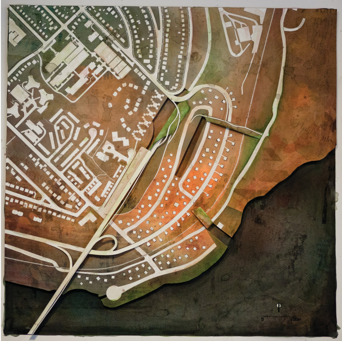
Paper site plan illustrating land re-stitching through off-ramps, homes, land bridges and bike network.
