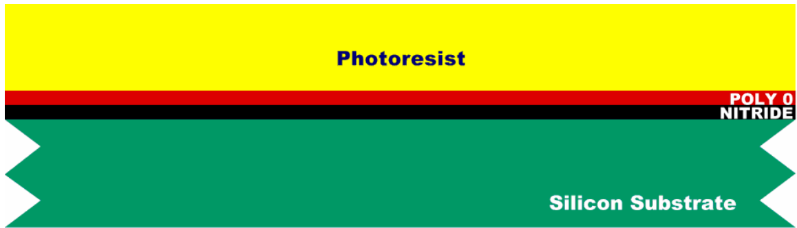
Figure 2: First Step of the PolyMUMPs Process: Deposition of Poly0 and Photoresist (Memscap [7])
