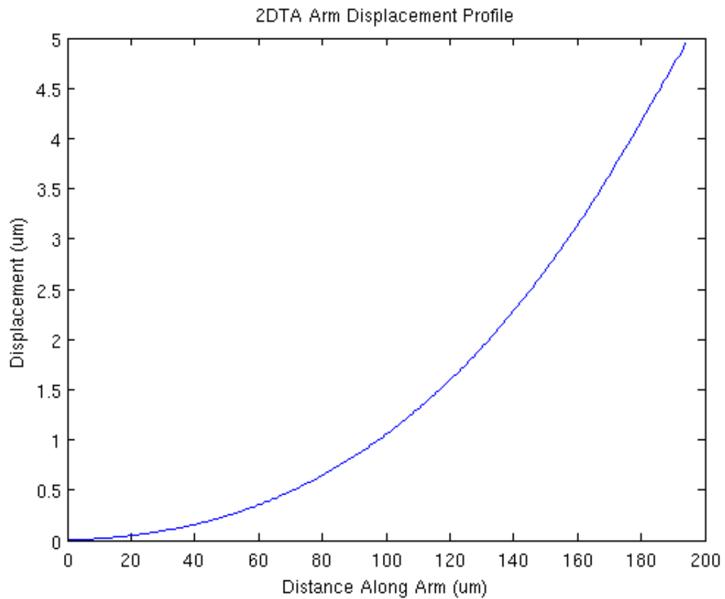
Figure 31: FEA 2DTA Displacement Profile along a Poly1 Arm
