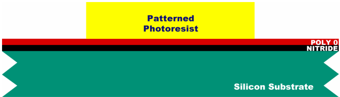
Figure 3: Patterning of the Photoresist in Preparation to Etch Poly0 (Memscap [7])
