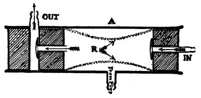
tubes, and space surrounding "R" be entirely filled with fluid, as air bubbles, being compressible, render the pump inaccurate.
