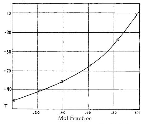
The solutions were cooled with a mixture of solid carbon dioxide and ether, so arranged that it could be evaporated under reduced pressure, and temperatures as low as —105°C obtained.
