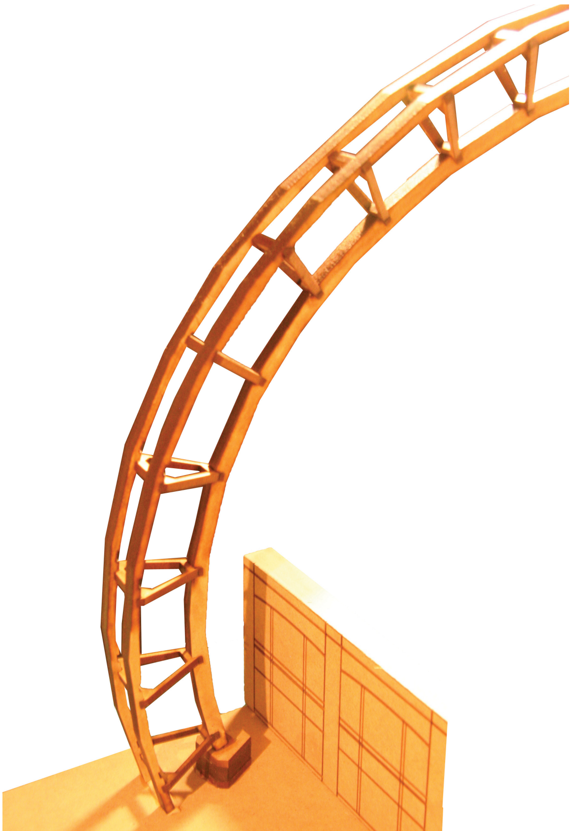
Model of one structural member of the superstructure and its distance from the armature.
