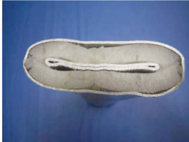
Figure 2.14. Collapse cross-section of an aluminum SP system [2.5].
