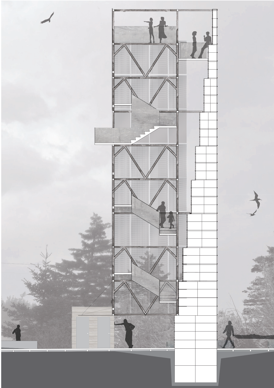
Section through Tower. At approximately 36 feet above sea level the path of the stairs pierces the cladding and presents the town of Whitehead. Finally, upon reaching the top of the tower, views towards the best kayaking areas are framed through the extension of the stereotomic tower and tectonic frame and cladding.
