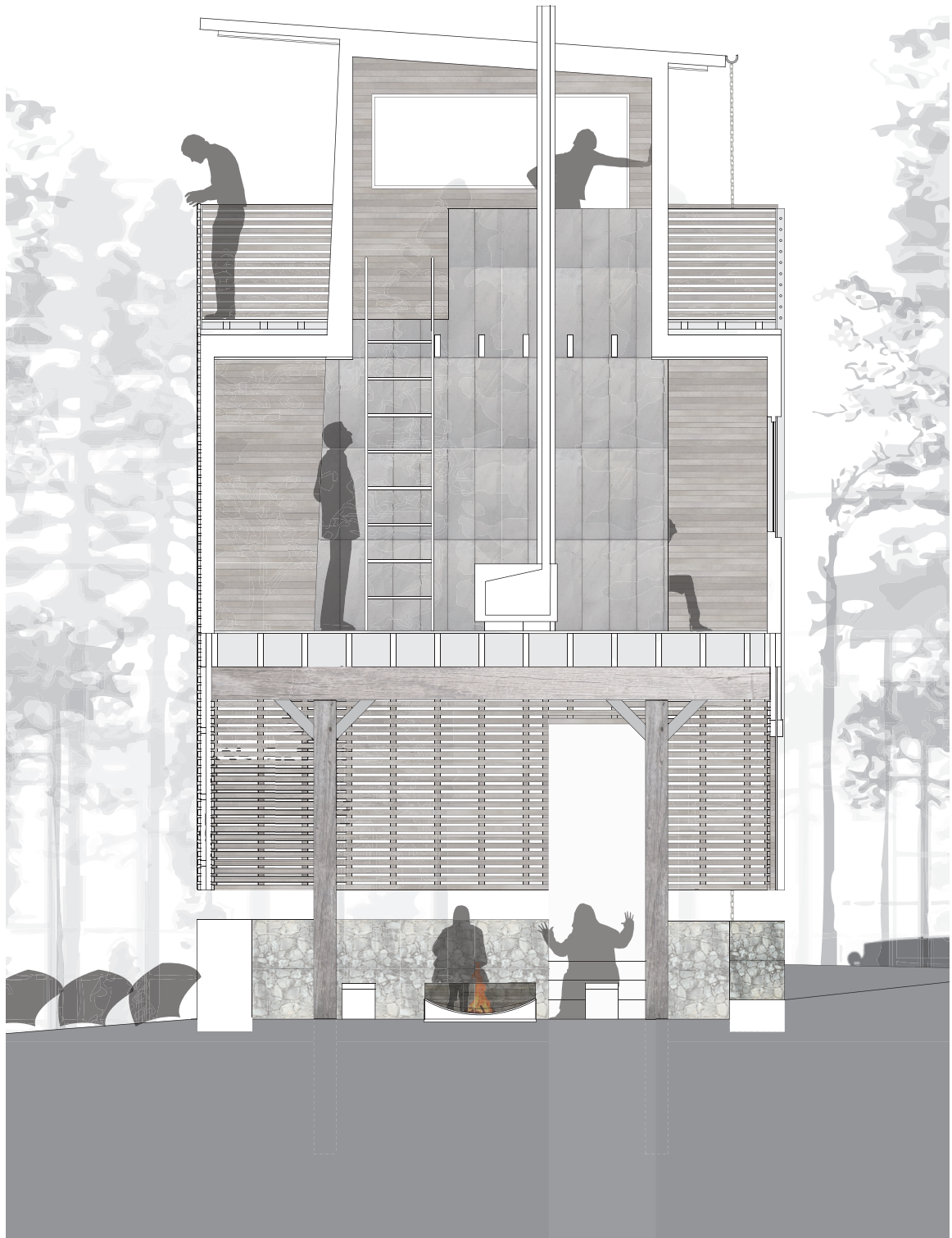
Section through Island Shelter. Above the drop beam construction, a platform framed structure provides housing for the night. Steel u-channels hang from the upper framing to provide a primary structure for the lightly constructed screen that encloses the ground level forest pavilion.
