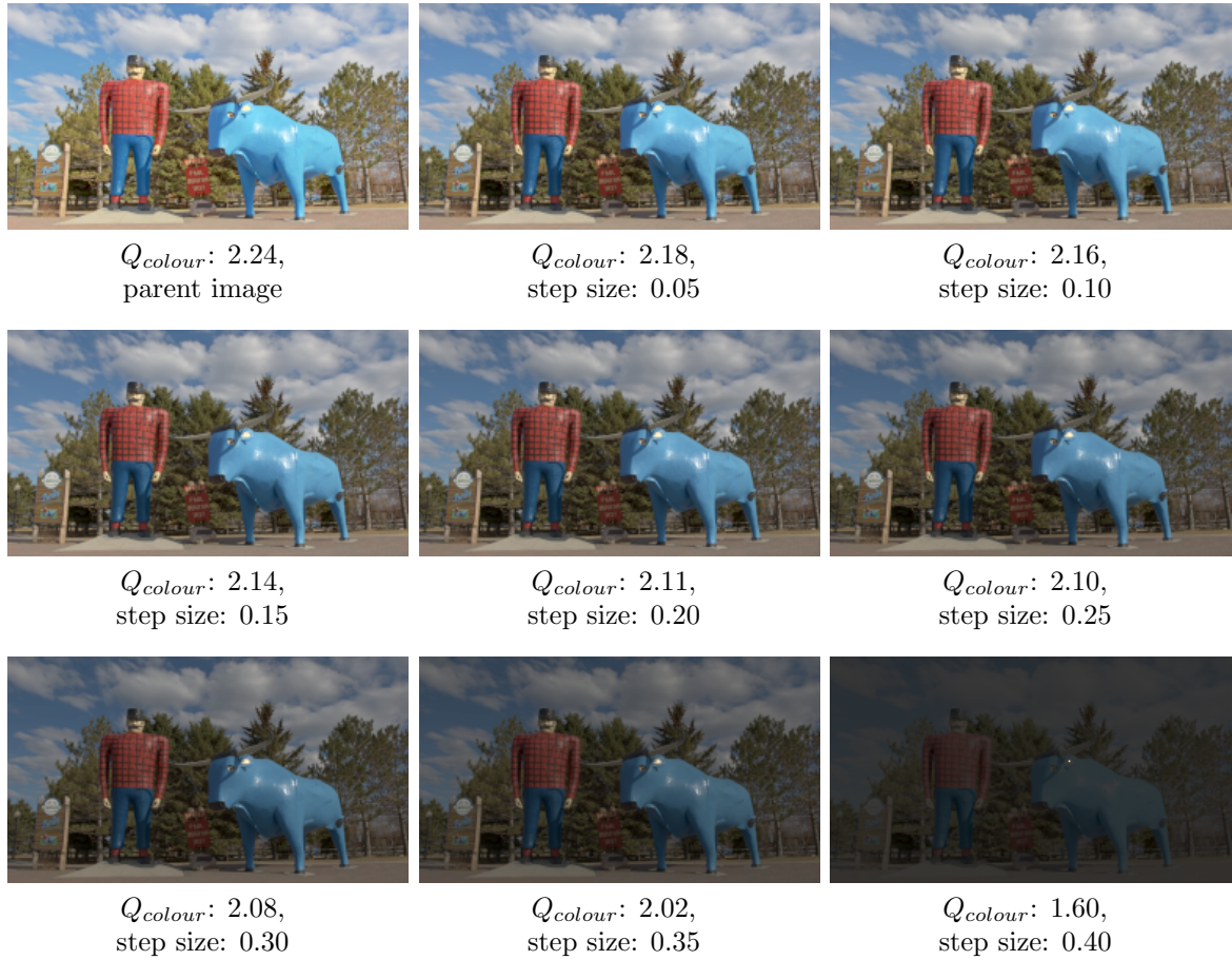
Figure 3.3: This series of images shows how the similarity metric Q_{colour} behaves with respect to step size. The images here are the result of fixing a single random direction in parameter space and then generating an image at increasing step sizes. In this case we see that the further along the direction we travel away from the image the metric decreases.
