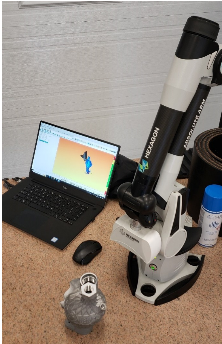
Figure 66: Laser scan setup of the AM heat exchanger
