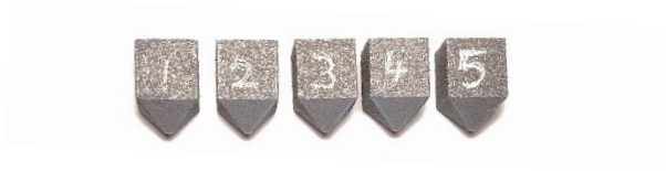
Figure 22: AlSi10Mg Density Specimens
