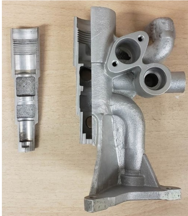
Figure 28: Sectional cut out of the thermal regulating valve area
