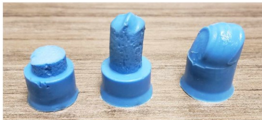
(a) Negative molds of the inlets and outlets
