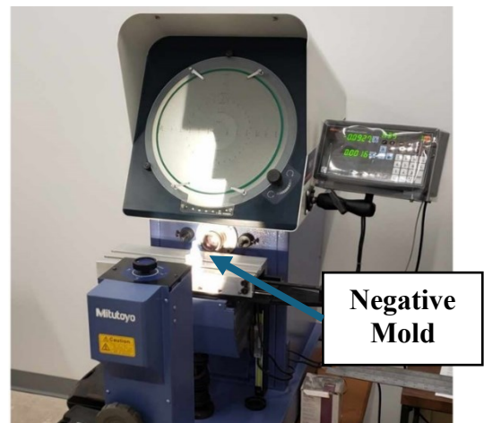
(b) Negative mold in the profile projector machine
