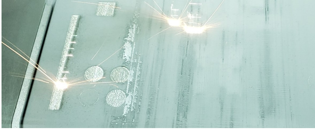
Figure 13: Effects of agglomeration on a spread layer of powder in an LPBF system
