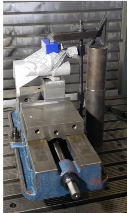
Figure 63: Machining setup 2 fixturing
