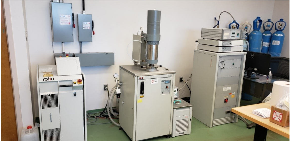
Figure 20: Netzsch LFA 427 system
