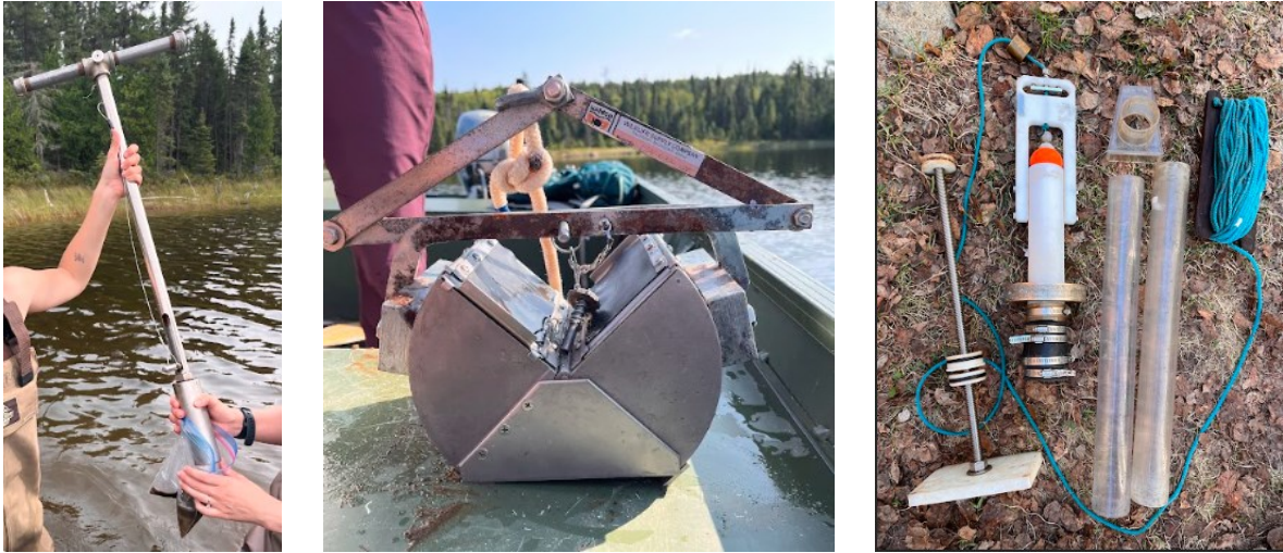
Figure 3.5 Sample collection methods: T-bar vacuum corer (left), Petite Ponar® grab sampler (middle), and NLA gravity corer (right).
