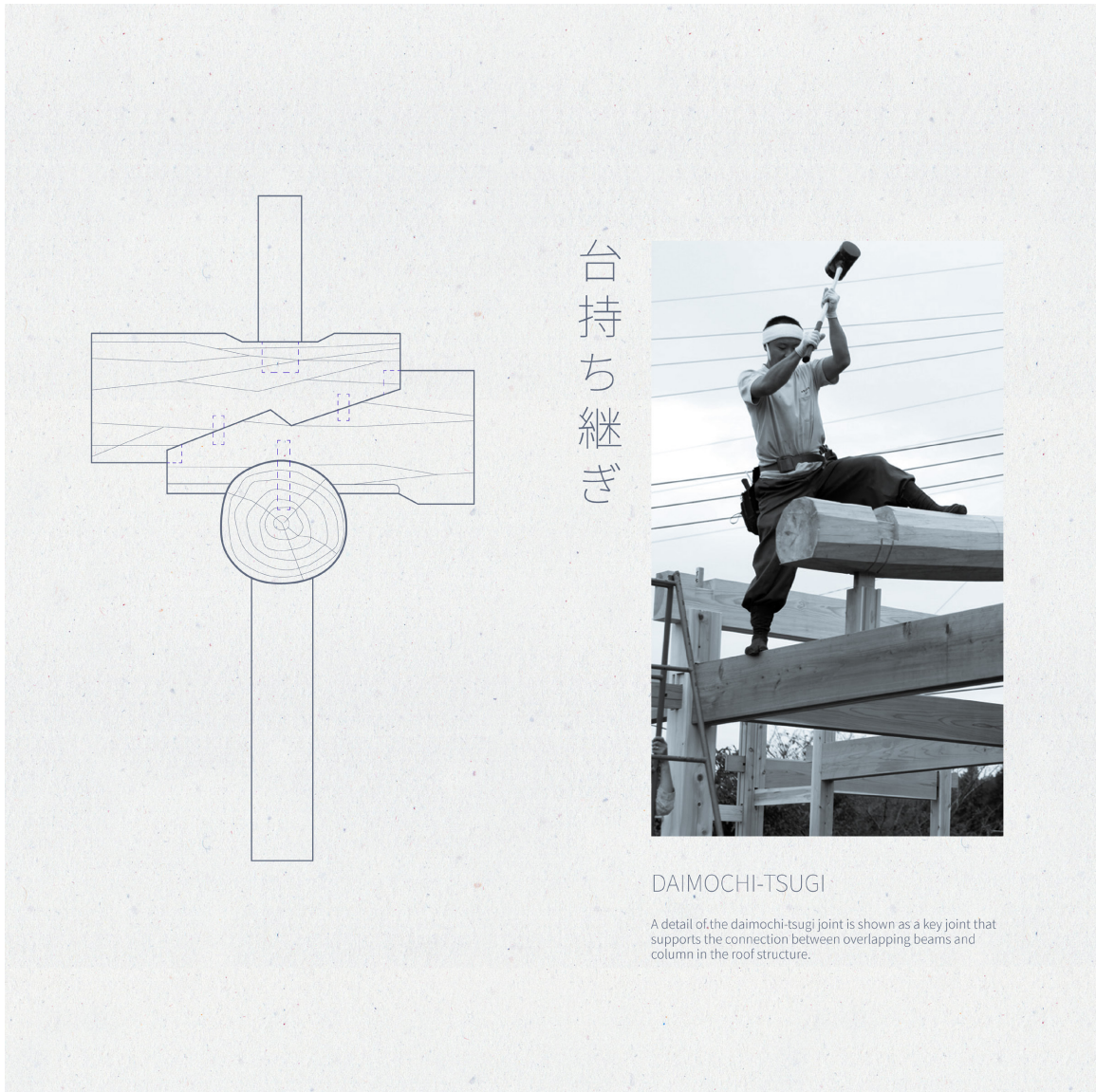
Machiya craftsmanship detail: Traditional wood assembly joint between column and overlapping beams
