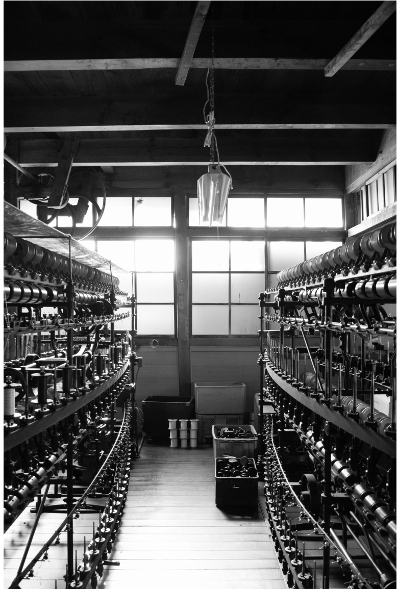
Atmosphere and lighting conditions of a silk workshop visited in Yosano, Kyoto, where silk thread is spun in preparation for weaving. The workshop is primarily lit with natural light diffused by frosted glass which was common across all workshops visited.
