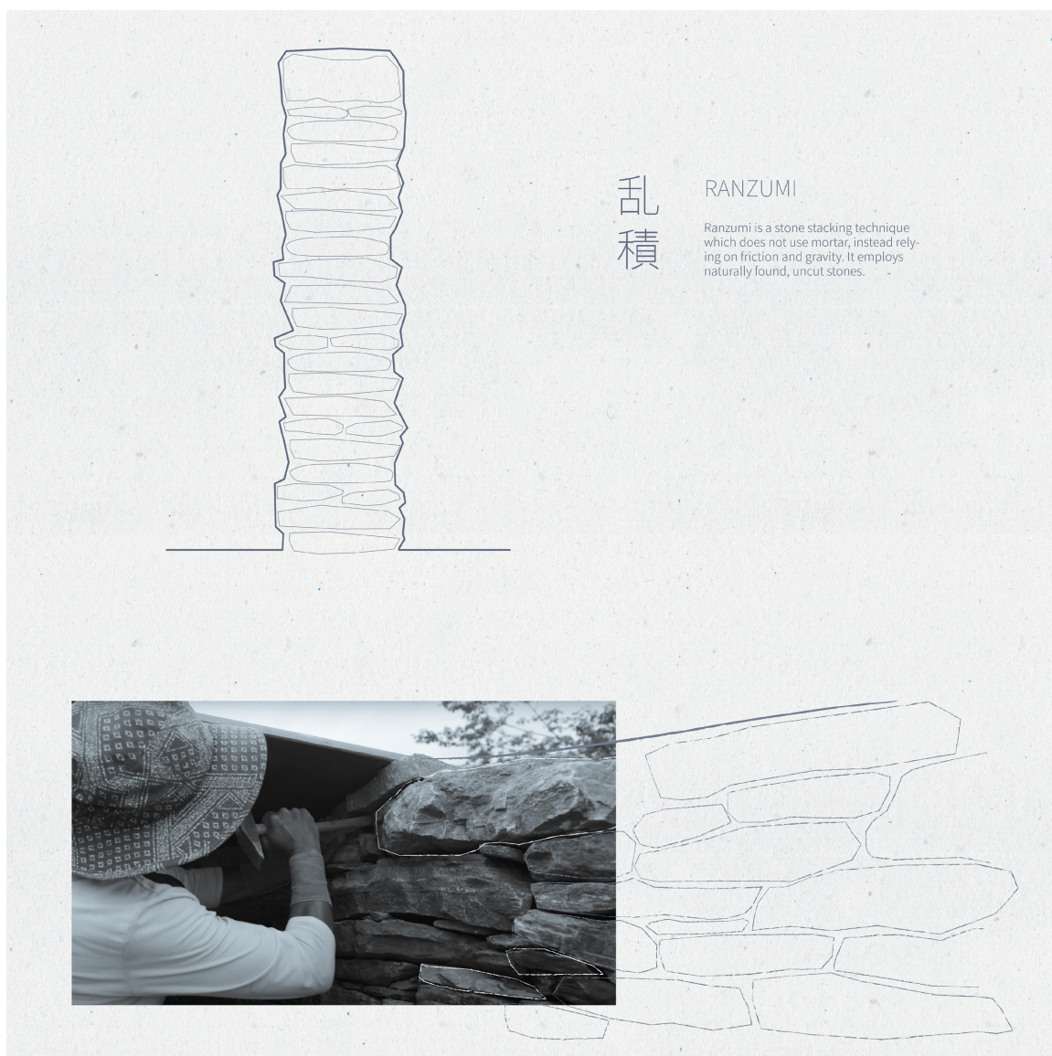
Craftmanship detail of the stacked stone garden walls
