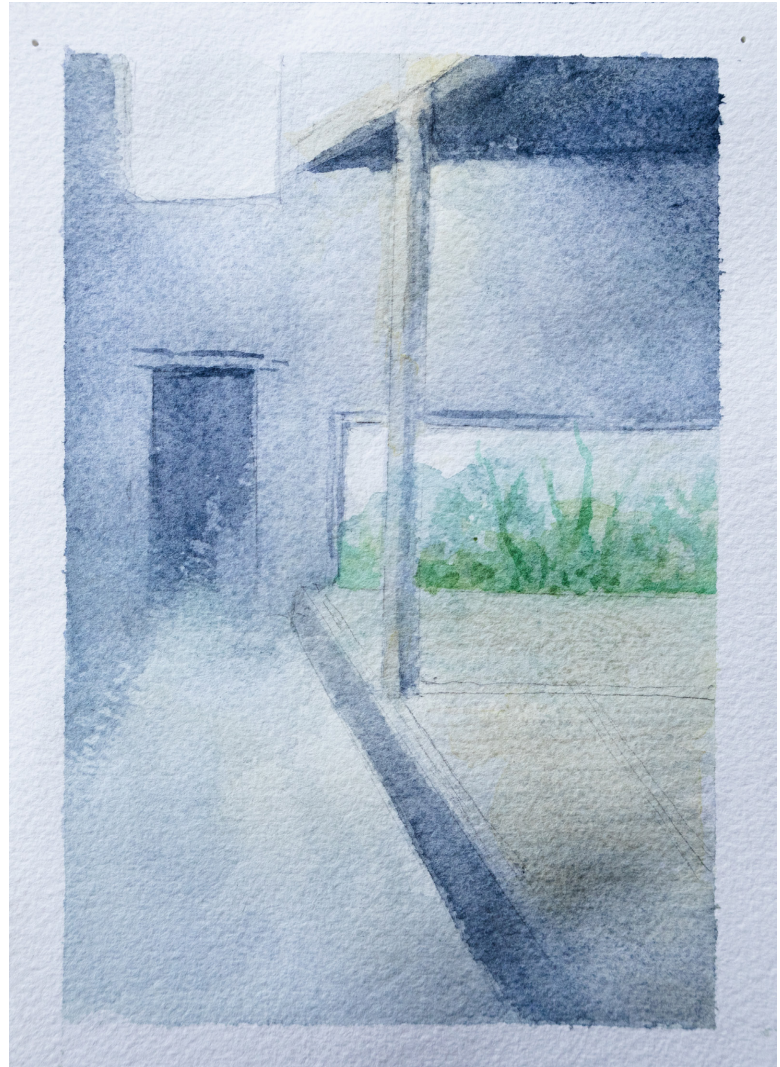
The atmospheric experience from the machiya's toriwa. Natural light permeates from the skylight at the top of the double-height toriwa. The floor of the toriwa is made from compacted earth, while the tatami mat area on the right is elevated.
