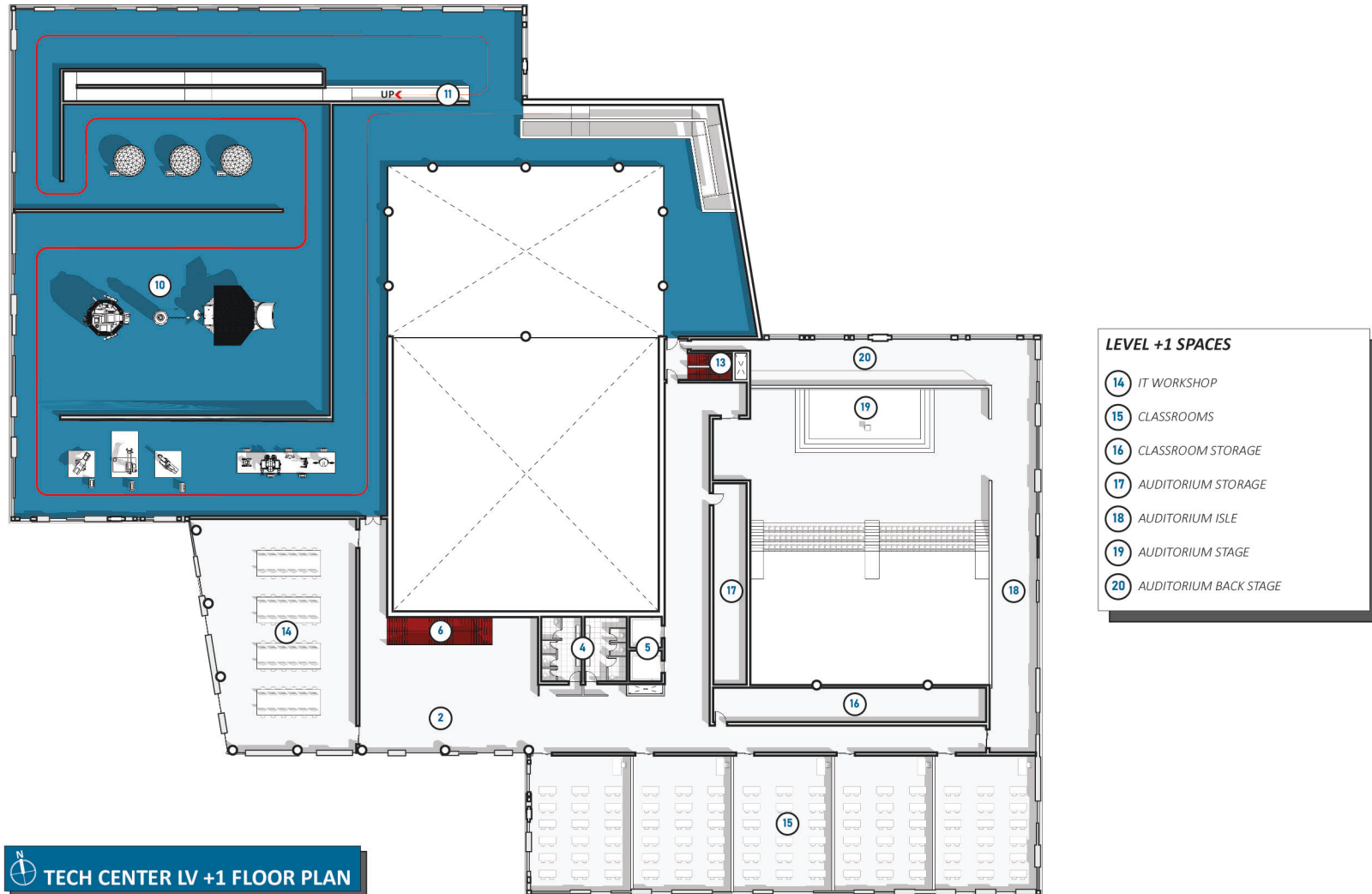
Figure 71: Level 1 floor plan of the Tech Center with the different public and institutional programs and the circulation path of the exhibition space.
