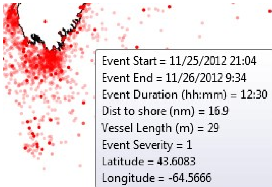
Fig 3.10 Zoomed in map view showing the geo-reference position of incidents plotted as bright red circles with the opacity determined by Equation 1. Hovering the mouse pointer over each geo-referenced data point provides the detailed summary of the incident, as in the example reproduced here.
