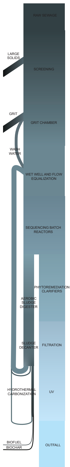
Proposed wastewater treatment plant process from R.V. Anderson Associates (2021) with biochar and phytoremediation additions.
