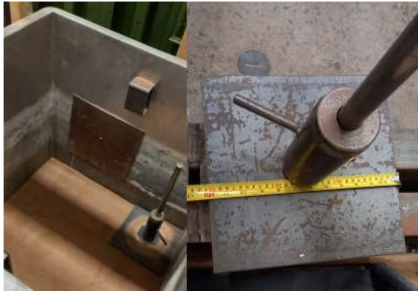
Figure 4-7 tamper for compaction bed sandy soil
