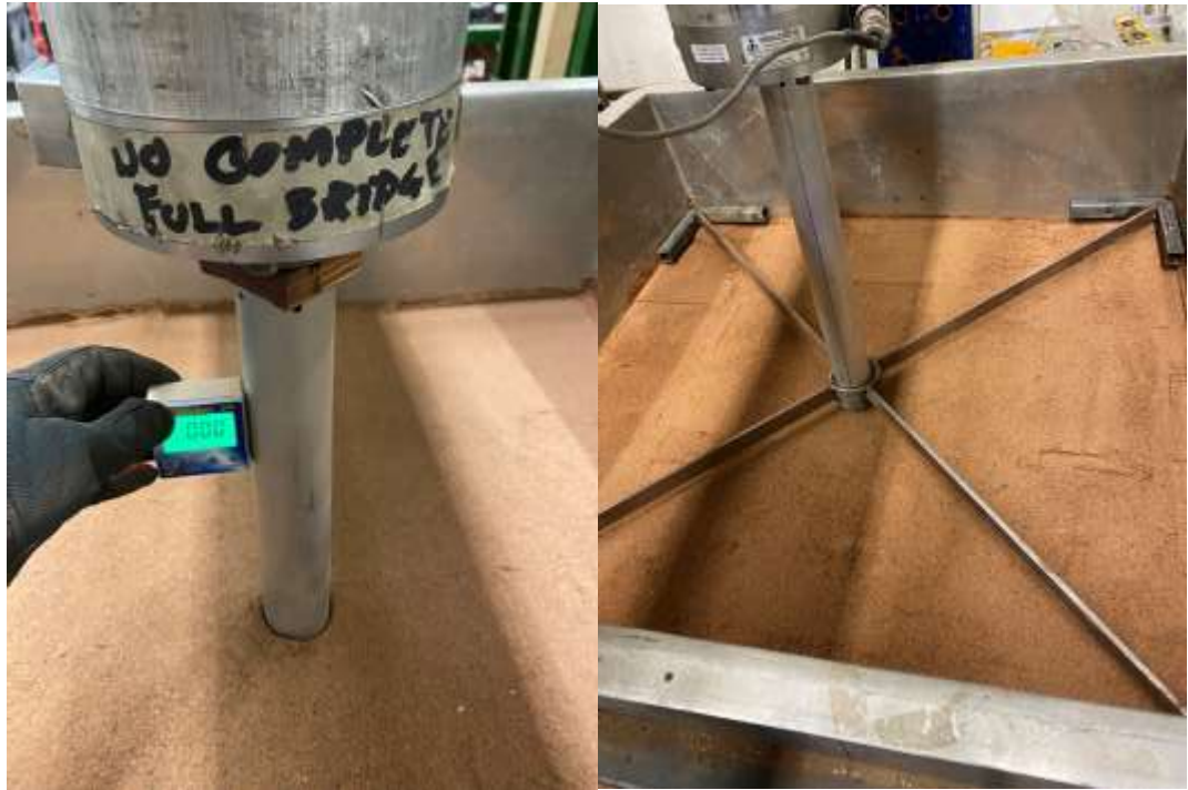
Figure 4-8 Placement of Tube in Soil
