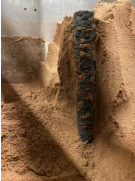
Figure 4-11 Bulging of the Stone Column After Loading
