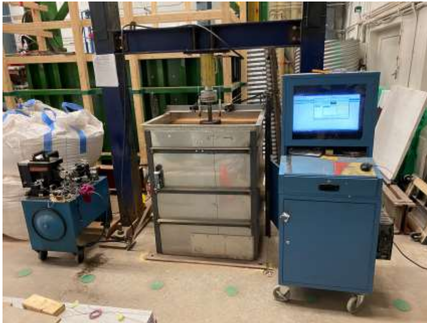
Figure 4-1 Test Box with hydraulic jack and DAQ
