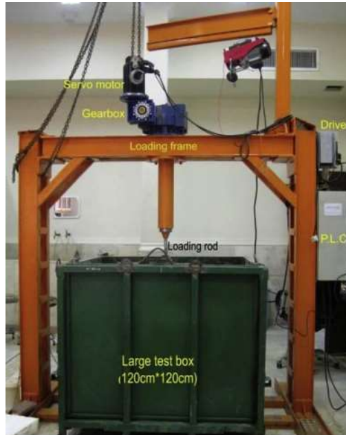
Figure 3-22 shows an example of a vertical loading test on stone columns [33].
