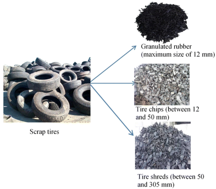
Figure 2-3: Sustainable utilization of scrap tires for geotechnical applications: Scrap tires being processed into TDA through cutting into various sizes
