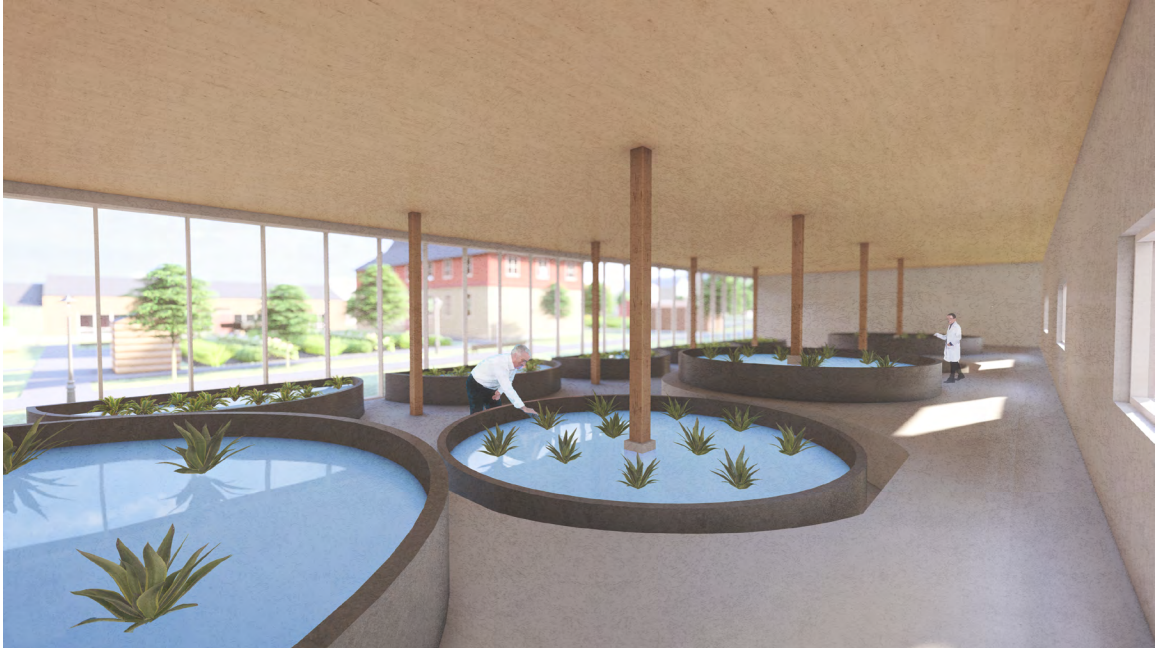
Rendered view of the aquaculture facility. Tanks of fish with floating plants allow the two to benefit from their mutualistic relationship. Tanks are placed at different elevations to prevent cross contamination.
