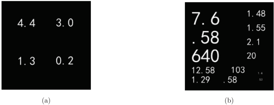
Figure 5.2: Generated Images using SuperTML: (a) Image Generated using SuperTML_EF on Iris data with equal importance given to each feature; (b) Image Generated using SuperTML_VF on Wine data with varied font size based on feature importance.
