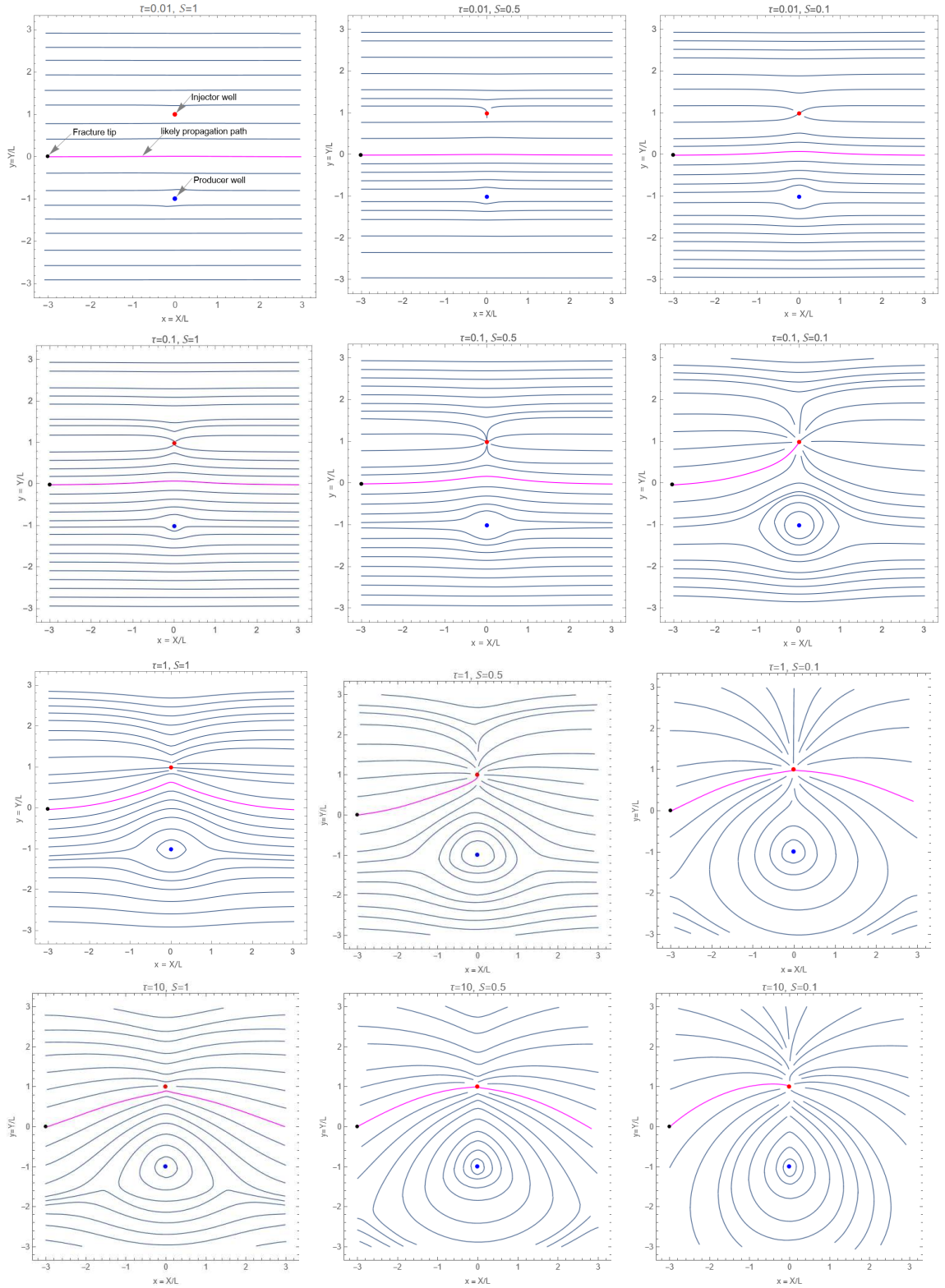
Figure 4.2: Maximum principal stress trajectories around an injector-producer system at various values of \tau and S
