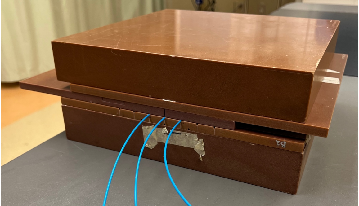
Figure 30: Photograph of assembled planar phantom, catheters are blue and inserted into the phantom via the grooves
