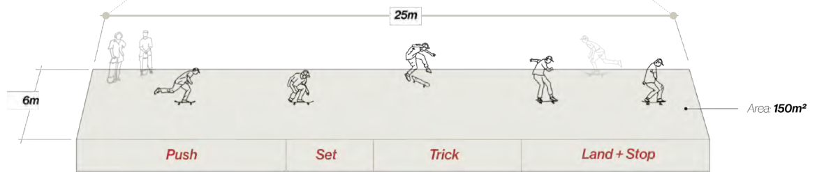
Network Hub, building plan. Minimum 25m runs of covered skateable space form important design parameters which help determine form.
