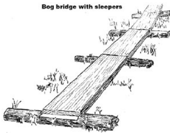
Bog Bridge With Sleepers (USDA 2007)
