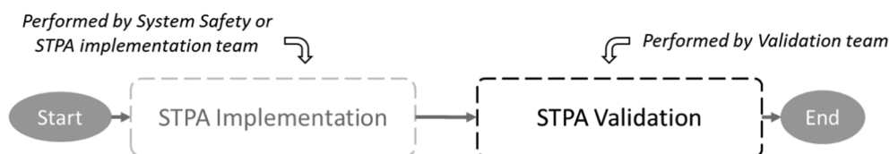
Fig. 5. Performing validation using the STPA validation framework after STPA implementation.
