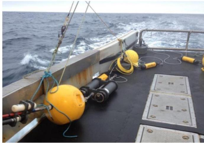
Figure 4: Mooring setup prior to deployment (reproduced from Delarue et al, 2018). Closest to camera is the fiberglass mast including tracking and flashing beacon, the yellow ball is a syntactic float, the double barrel black cylinders are the hydrophone and battery packs followed by 20 m of yellow rope, acoustic release assembly, and at the starboard quarter, an anchor assembly consisting of 5 or 6 Olympic weightlifting plates depending on shallow or deep-water mooring configuration.
