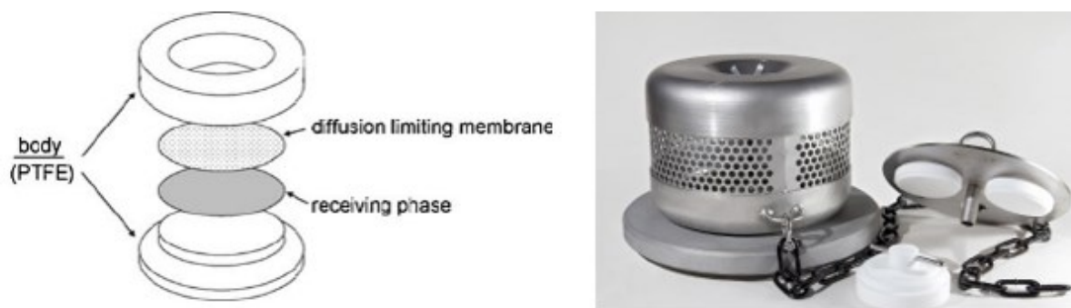
Figure 2. General configuration of the chemcatcher and deployment kit. Labelled elements of the chemcatcher (left), adapted from Ahkola et al (2012). Chemcatcher deployment kit (right), adapted from Chemcatcher (2022).
