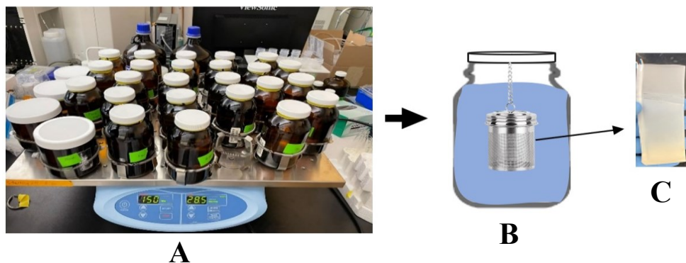
Figure 6. A bench scale setup for the extraction of geosmin and 2-MIB from spiked DI and lake water matrices. A. a batch of samples stirring on an orbital shaker; B. a stainless-steel casing contained an adsorbent immersed in the spiked sample; C. a pre-measured mass of adsorbent inside a heat sealed nylon bag
