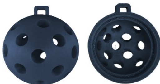
Figure 4. COVID-19 sewer cage (COSCa) passive sampler (external and internal view). Adapted from Hayes et al (2021).
