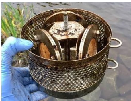
Figure 1. Polar organic chemical integrative sampler (POCIS) retrieved from a lake after 28 days of exposure time. Adapted from Brophy (2019).
