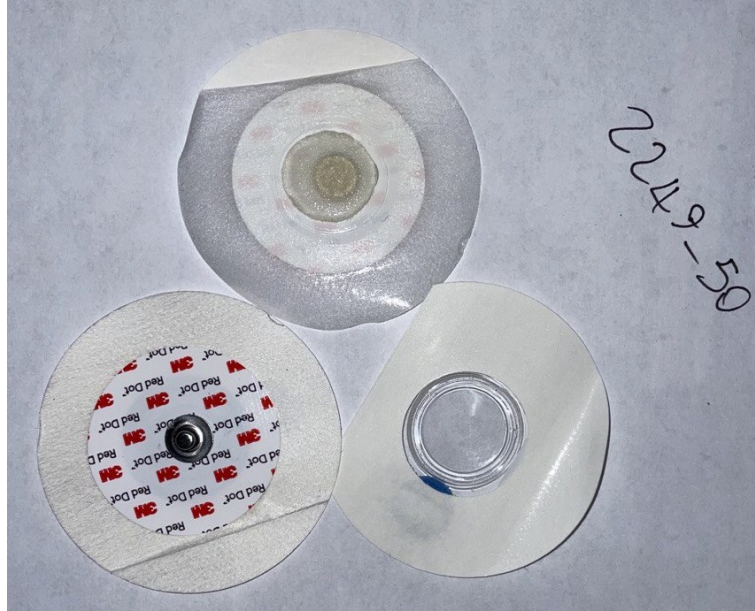
Figure 15: 3M RedDot 2249-50 ECG electrode - Ag/AgCl with sponge
